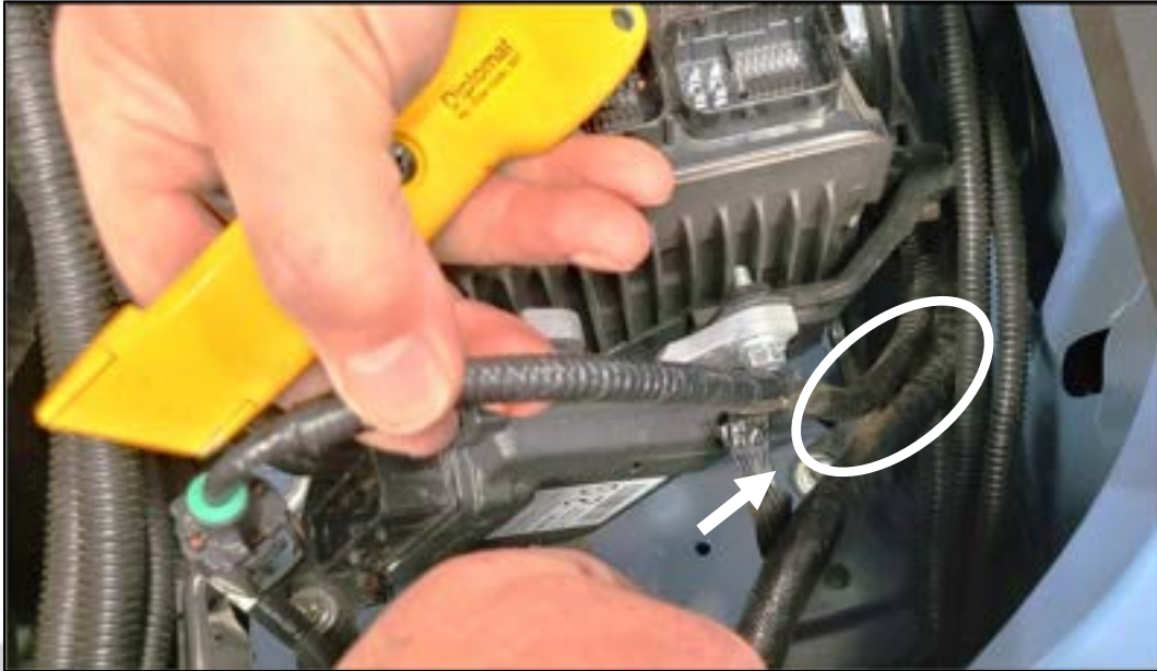
Figure 7. Cut tape to allow harness separation
