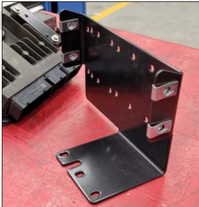
Figure 12. Correct U-nut orientation
