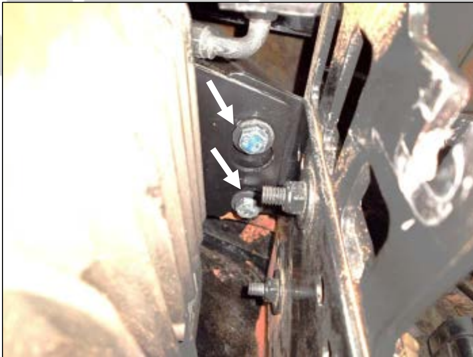
Figure 18. Ensure that the bracket is fully engaged with the fasteners
