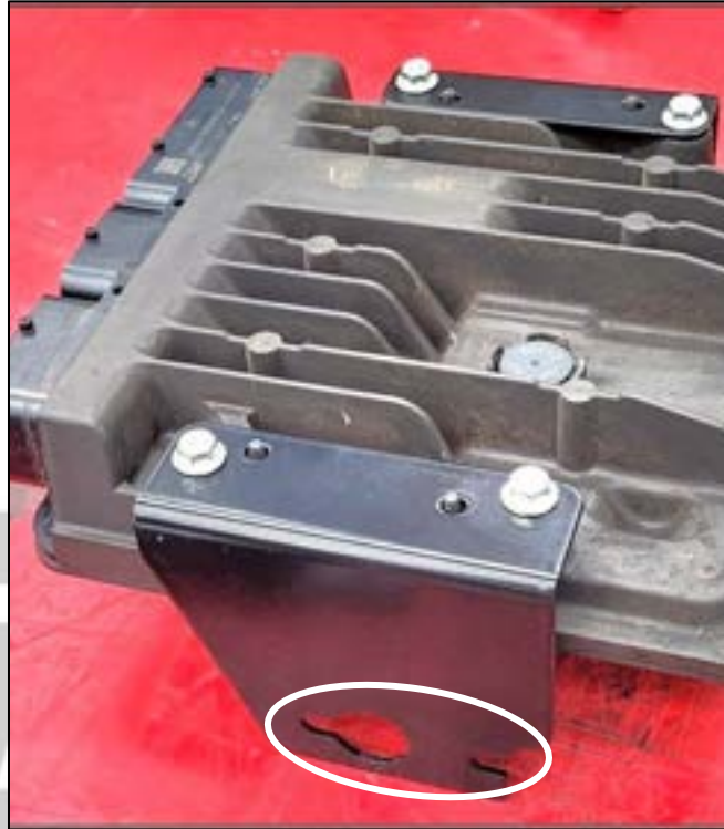
Figure 11. Correct orientation of ECU brackets
