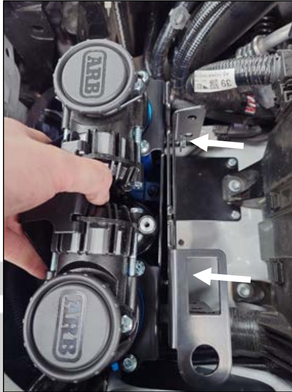
Figure 28. Hold brushed compressor in place
