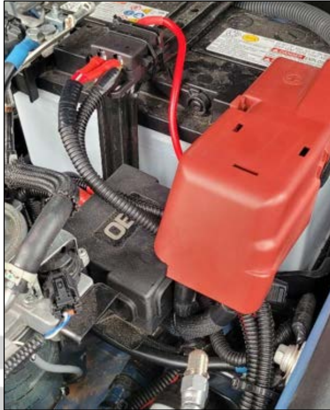
Figure 43. Recommended mounting location for compressor fuses
