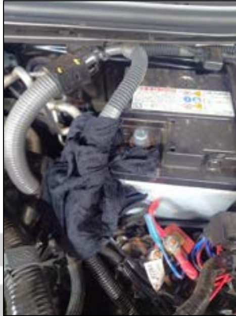
Figure 3. Negative Battery terminal disconnected and wrapped with a rag
