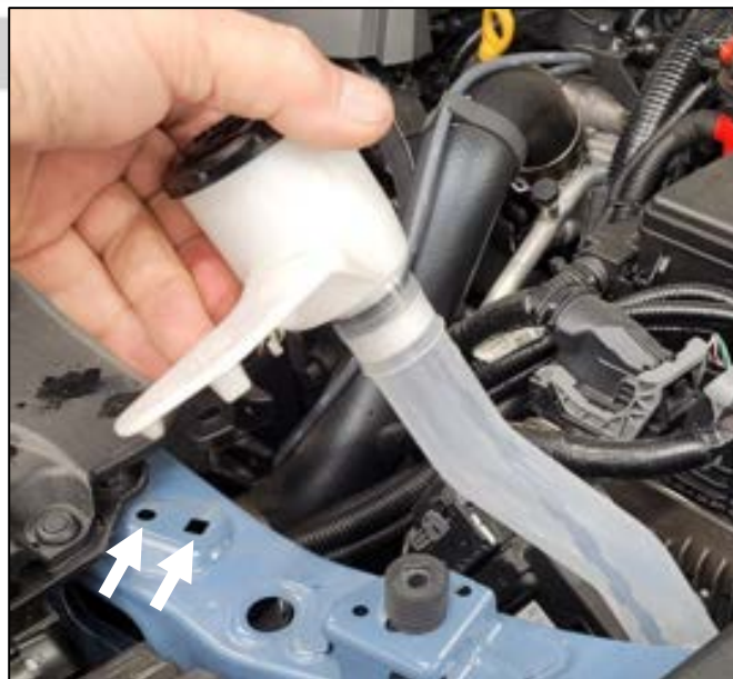
Figure 4. Remove washer fluid fill tube
