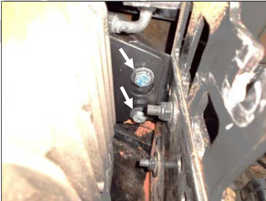
Figure 30. Ensure that the bracket is fully engaged with the fasteners
