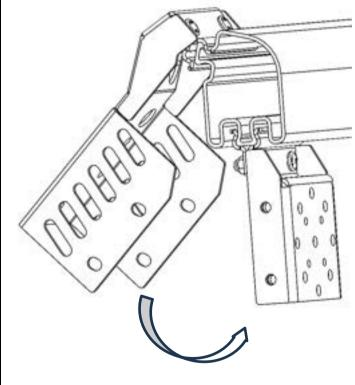
2. Install the assembled mount to the dovetail, centre with the single mount and rotate to align.
