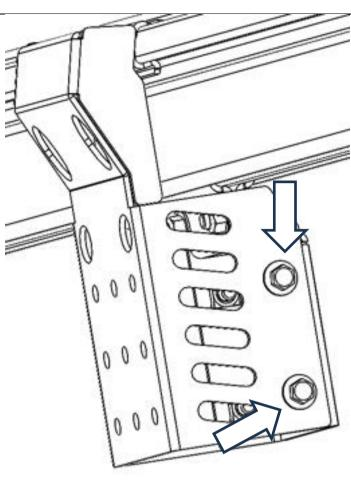
3. Install four M8 x 20 FL bolts, two per side, and tighten to be firm.
