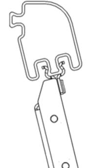
1. Using the 6582535 mounting bracket as a template, drill Ø8.5mm holes in each corner. Remove brackets and deburr all holes.
