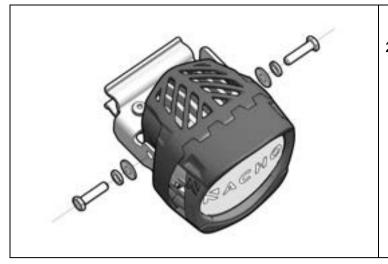
2. Assemble brackets onto the Nacho Quatro light, using the 1/4-20 hex bolts, lock washers and flat washers provided with the light, as shown.
