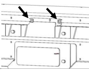
34. Install two snap in grommets into the square holes on the front of the bull bar as shown.
