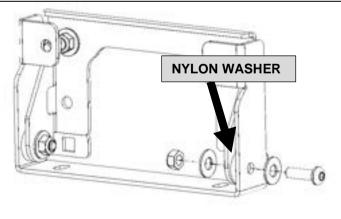
30. Attach the radar bracket to the mounting bracket using two M6x20mm button head screws, four 16mm M6 washers, two M6 nyloc nuts and two 20mm nylon spacers.
