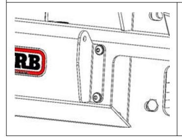
44. Fit left and right number plate mount brackets from the winch fit kit using M6 screws, washers and flange nuts provided. Leave screws finger tight at this stage.
