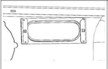
Install Nylon plugs (6821116). (4 off) Into Clearance Light/Turn Signal Brackets. (RH Shown).
