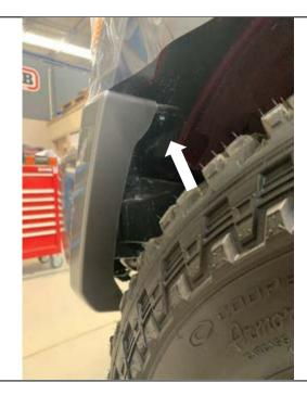
3. Remove two nuts from the corner of the bumper cover under each wheel arch.
