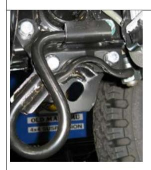
Refit the tow hook/s to the vehicle 52. using the original bolts removed in Step 10. Fit tow hook spacers (i.e. two 4mm thick washers 4581011) between the tow hook/s and each chassis rail/s for the two lower bolts.
