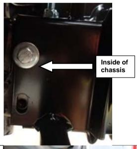
49. Align the mounting holes and fit two M12 x 170mm PC11.9 (2016+ single cab variants) or M12 x 140mm PC8.8 bolts with M12 flat washers through the chassis from the bottom. Fix with M12 flat washers, and nyloc nuts.
