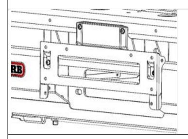
43. Fit number plate bracket using two M6x16mm button head screws, two M6 serrated flange nuts and two M6x12.2x1.2 flat washers.
