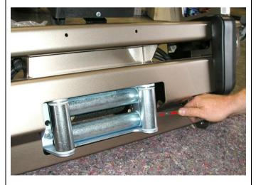
33. Fit roller fairlead into cutout and refit bolts and tighten firmly.
