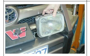
54. If fitting optional driving lights to vehicle do so at this stage. Guide ratchet spanner between the upper and lower pans, as shown, to tighten the lights to the bar.
