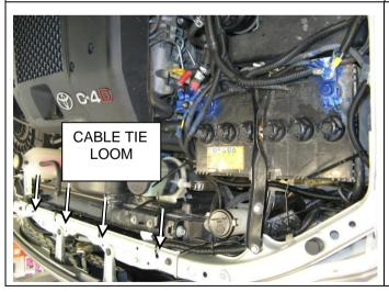
19. Using the cable ties supplied, secure the loom being sure to keep clear of any hot, sharp or moving surfaces.
