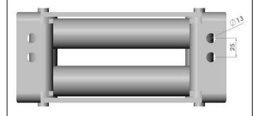
32. Drill two new Ø13mm holes in the roller fairlead provided in the kit, as shown on the adjacent picture.
