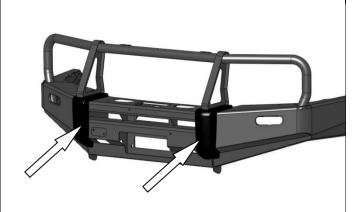
20. Fit the buffers to the bull bar using the 6mm flange nuts provided.
