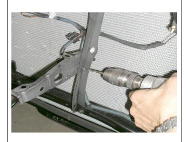
5. Remove the protruding bracket in front of the radiator, as it is no longer required (note: the vertical member of this bracket must not be removed as it holds the bonnet latch in position). This may be done by either drilling out the existing spot-welds with a 5mm drill as shown, or by cutting it off with a grinder. Re - locate the air temp sender (if fitted) to one of the holes in the vertical bracket.
