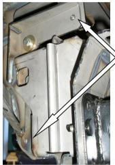
41. Once satisfied with the position of the bull-bar, using a Ø10mm drill, drill through the Ø10mm holes in the impact absorber, 2 holes per side, and secure using the M10 x 1.5P x 30 bolts, two flat washers per bolt, spring washers and M10 x 1.5P hex nuts.
