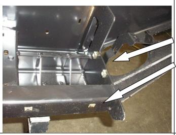
21. Fit cage nuts and nylon plugs to the bull-bar.
