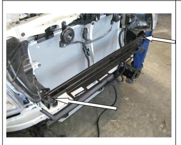
6. Fasten the lower grill bracket to the vehicle head lights, as shown, using M8 x 25 black bolts, flat washers, spring washers and flange nuts.
