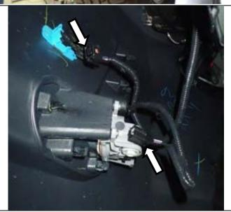
If equipped, disconnect fog light wiring and front parking sensors – (Right Hand side shown).
