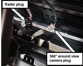
8. If vehicle is equipped with Toyota Safety sense and/or 360° around view camera, locate the plugs (positioned behind the badge on the grille) and unplug from their respective units prior to proceeding.
