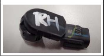
12. Using a paint pen or white marker, label each parking sensor (Left or Right) prior to removing from bumper.
