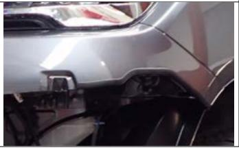
46. Fit Pinch weld to RH side along the full length of the cut edge. Carefully trim off any excess length and use remainder for other side.
