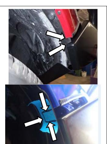
97. Use a pair of shears to cut a section approximately 20mm x 20mm from the inner guard outer edge to allow it to be pushed into the end of the wing. (RH Shown).
