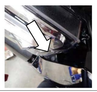
5. Remove all fasteners and scrivets retaining bumper along inside edge of wheel arches – (Right hand side shown).
