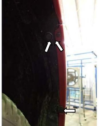
Remove all fasteners and scrivets retaining bumper along lower lip – (Left Hand side shown).
