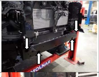
15. Remove two M10 bolts on both sides (4 total) fixing crash beam to chassis and remove crash beam.
