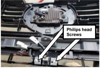
13. If equipped, remove the camera and camera bracket by removing the two Philips head screws connecting the bracket to the grille.
