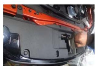
100.e-install upper radiator cover panel and fasten using eight OE scrivets.
