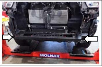
Remove plastic lower crush absorber from vehicle and discard.
