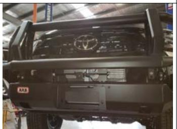
76. Check the clearance of the bar to the vehicle, and adjust position of bar left/right until it's sitting central to body, then tighten all fasteners joining mount assembly to chassis brackets (four M10 ARB and two M10 OE bolts each side).
