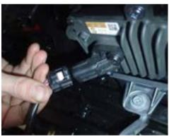
45. If vehicle is equipped with adaptive cruise control, reconnect radar.
