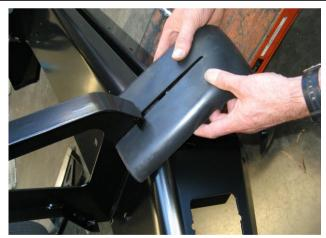
64. Carefully slide top section of buffer past edge of cover strap as shown
