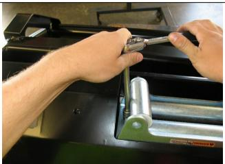
56. Fit the roller fair lead, pull only the end of the cable through and adjust the position of winch then bolt up securely. Use the 1 ½" long bolts in the top and 1 ¾"in the lower set through the RFL.
