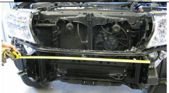
71. Tap the outer flange of the mount brackets until they are hard up against the tow hook mount area. Nip up the lowest outboard nut on each bracket. Brackets should be about 935mm apart
