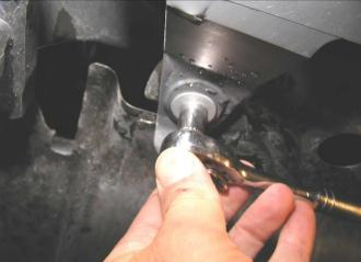
6. Remove lower bumper retaining screws.
