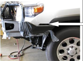
70. Ensure the bull bar is sitting on the vehicle level and the gap between the bumper bar cut and the bull bar wing is even.
