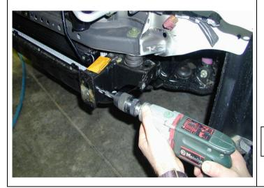
33. Using a power drill with Dia13mm bit, drill out captive nut in hole immediately behind chassis flange as shown, for both RH and LH chassis ends
