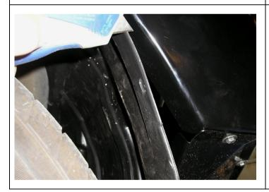
90. If required, trim the outer edge of the fender liner as shown so that it will clip in behind the wing with the maximum grab
