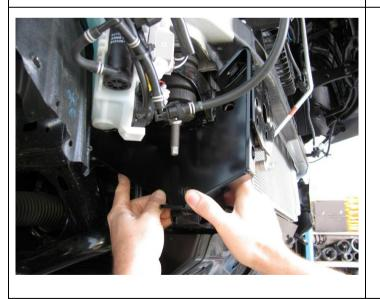
38. When the RHS side brace are fitted in position as shown, insert <u>fine thread M12</u> <u>x1.25P x 30 bolt</u> and washer sets into lowest hole position to chassis. There is an existing captive nut in chassis, **but do not do up tight.**
