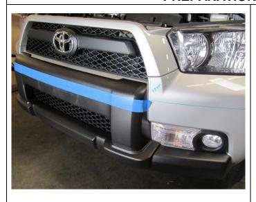
8. Temporarily apply some masking tape joining the cutting line positions from each of the bumper outer sections. Apply the tape so the top edge is on the cutting line
