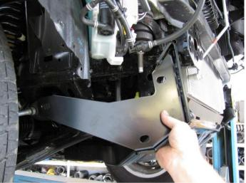
37. Fit handed specific side brace as shown, locating over the captive nuts at the rear of the chassis.
