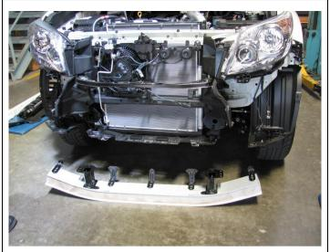
30. Remove reinforcing beam at mounts to chassis by undoing the M10 fine thread bolts. Set beam aside, it will not be reused
