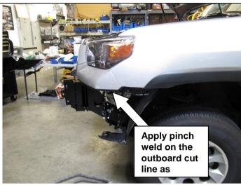
53. Fit bumper back onto vehicle and apply pinch weld to edges as shown
