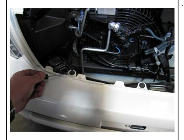
14. Remove the plastic rivets securing the top of the bumper
