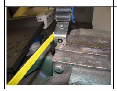
50. Modify the clamp plates for the power steering pipes by cutting off the flange as shown then drilling a Dia 8.5 hole 8mm from the bend as shown
