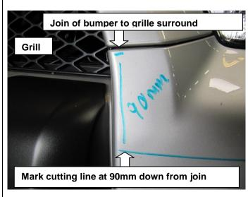
Mark a position for the cutting line at 90mm (3 ½") down from bumper to grille surround join inboard of headlamp as shown, repeat on other side of vehicle
