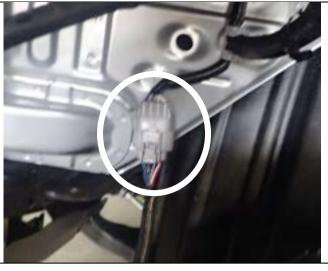
13. If fitted, disconnect the master plug for the front parking sensor loom. Located on passenger side in front of wheel.
