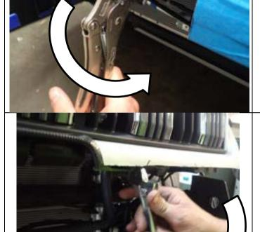
19. Using a set of vice grips or a shifter, bend the two sheet metal tabs backwards to increase winch clutch lever clearance.
