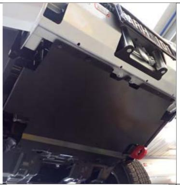
84. Attach the centre stone shield to the bar as shown using M8 hex bolts (5), and flat washers.
