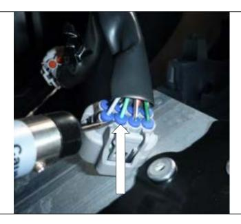
55. For GX models without LED headlights, loom 6821344 Is not required. Power supply for the clearance lights can be taken from the 8pin plug on the underside of the headlight as shown.
