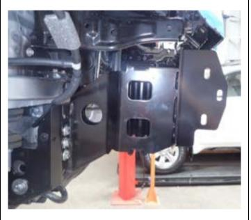
32. Fit impact absorbers to chassis ends using *fine thread M10 x 1.25 x 30 bolt* and washer sets supplied, note that the brackets are handed, slide them towards the centre of the vehicle on the adjustment slots *do not do up tight. (4 per side)*
