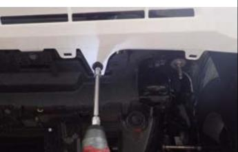
14. Remove all bolts and scrivets from below the lower section of the cut bumper.
