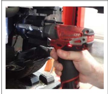
22. Remove crash cans from chassis by undoing the M10 fine thread bolts. (4 per side)
