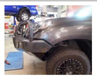
67. Once the bull bar is positioned and the clearance/gap is 18-20 mm, tighten all the mount bolts to specified torque.
