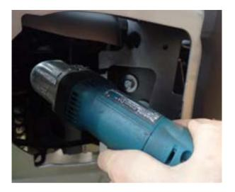
68. Using an electric drill and a Ø10.0 mm drill bit, drill two pinning bolt holes through the bull bar upright each side using the holes in the mount bracket flanges as a guide.
