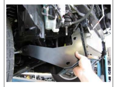
28. Fit handed specific side braces as shown, locating over the captive nuts at the rear of the chassis.
