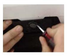
15. Remove lower screw from inside of each wheel arch which holds lower bumper section to vehicle.
