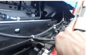
12. If fitted, cut all clips holding head light washer lines to lower section of bumper with side cutters
