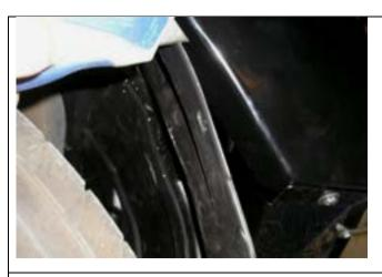
80. Trim the outer edge of the wheel arch liner as shown so that it will clip in behind the bull bar.
