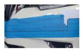
11. Using a jigsaw or multi-tool carefully cut along the marked edge.
