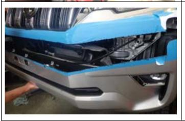
16. Ensure all Head Light Washer lines are free from lower section of cut bumper and the parking sensor loom has been disconnected. Remove lower cut section from vehicle.
