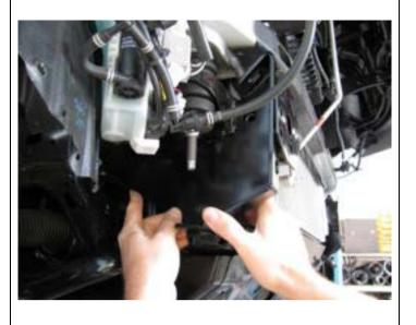
29. When side braces are fitted in position, insert fine thread M12 x1.25x30 bolt and washer sets into lowest hole position to chassis. There is an existing captive nut in chassis, but do not do up tight.
