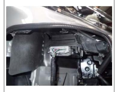
53. Power supply for the indicator circuits can be taken from the large connector under the head lamps. Rotate the grey lock downwards and disconnect the connector for ease of access.
