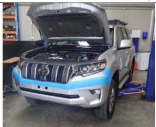
5. Apply wide masking tape along bumper as shown.
