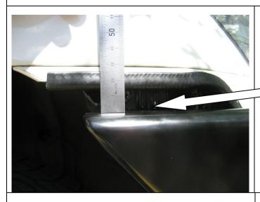
67. Ensure the bull bar is sitting on the vehicle level and the gap between the bumper bar and the bull bar wing is parallel.
