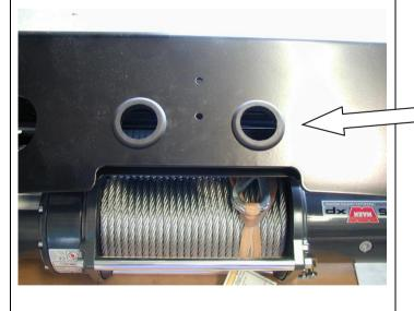
59. Insert the two rubber grommets into the top face of bull bar.
