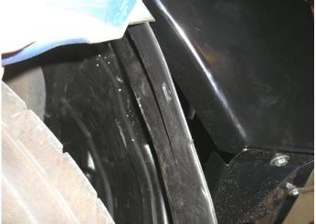
86. Trim the outer edge of the fender liner as shown so that it will clip in behind the wing, then trim off the bottom of the liner flush with the lower face of the wing panel
