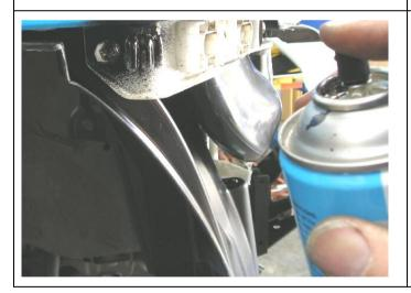
42. Spray front exposed face only of plastic bracket as well as any lower sheet metal in the immediate area visible when bull bar is fitted with black spray paint as shown and refit plastic bumper clip to vehicle
