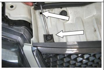
13. Remove the top panel and grille – for the grille prise out plastic clips along the top first, then pull outwards and upwards to release lower clip points along the lower section of grille attaching to top flange of the bumper
