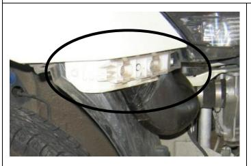
40. Remove plastic bumper clip both sides of vehicle
