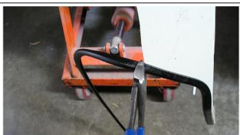
46. Remove tape, deburr cut edges with a file then apply pinch weld to side cut edges as shown and then trim off excess
