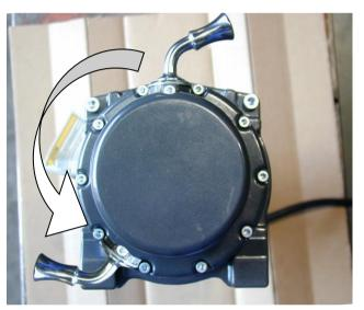
53. Remove the cap head screws retaining the gearbox to the winch drum. Carefully lift the gearbox a small amount (5 mm) and rotate144 degrees counter clockwise (four hole spacings) and re-fit the cap screws. This places the winch handle in the correct orientation.
