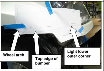
3. Fit the template to the RHS of the bumper aligning with the wheel arch, top edge of the bumper and the head lamp lower corner and tape in position
