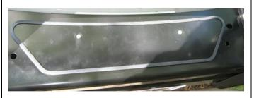
51. Fit panel to top face on bull bar using 2 x M6 dome head stainless steel screws, flange nuts and stainless steel flat washers.
