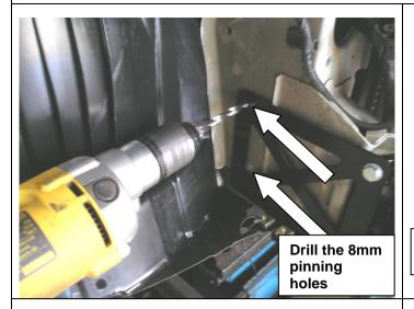
27. Using an 8mm drill bit, drill holes through the side of vehicle chassis using the top and lower rearmost holes in brace as a guide.
