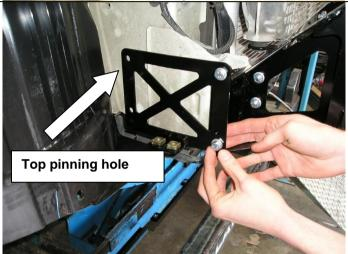
24. Fit side braces using supplied M8 hardware then fit M8 cage nuts to two lower positions as shown below
