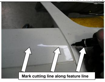
6. Mark the cutting line across the front of the bumper in line with the feature line and lower edges from the template.
