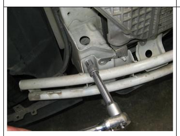
18. Remove reinforcing beam by undoing 4 x fastening nuts. Set beam aside, it will not be reused
