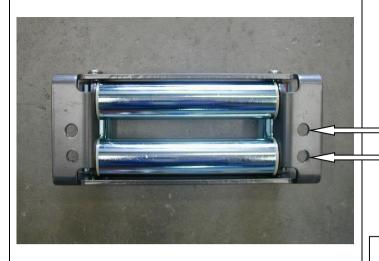
Using a 12mm drill bit, mark & drill two new holes in the roller fairlead 25mm below the original holes.
