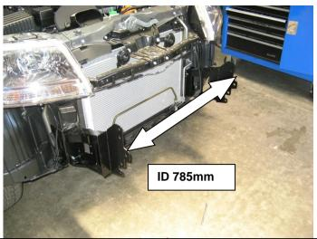
23. Measure inside dimension across mount flanges and adjust bracket side ways position so that there will be a slight amount of clearance to the bull bar uprights, (785mm) when bull bar is fitted later on. Once in position tension to specified torque
