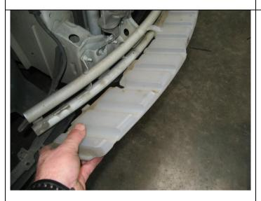
17. Remove reinforcing beam plastic impact buffer
