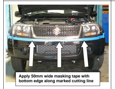
7. Apply masking tape with the bottom edge on the marked cutting line.
