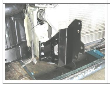
22. Fit mounting brackets using supplied brackets and nut and washer kits
