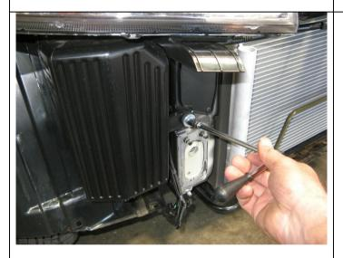
21. If fitted, remove air intake on the RHS of vehicle
