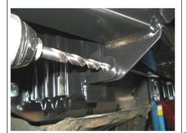
70. Using an electric drill and a 10.0 mm drill bit, drill two pinning bolt holes through the bull bar upright each side using the holes in the mount bracket flanges as a guide. One hole is located in the lower lug of the mount face and one up above the welded nuts. Use access through the light surround opening for the top hole.
