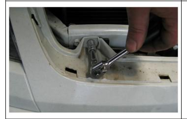
14. Remove bolts and plastic clips securing bumper to cross member.
