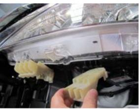
6. Remove the 2 plastic bumper retainer blocks from the underside of each of the head lights and discard.
