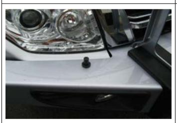
57. Fit Headlight Washers to bar if required, refer to Washer Kit Fitting Instructions **#3789274**
