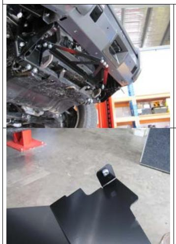
Attach the Winch Brace to both the bar and the mounts using 7 x M10 SEMS bolts and M10 flange nuts.
