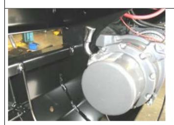
50. Position the winch with the mount face facing upward on an adjustable table or similar and with the assistance of another person lower the bulbar over the winch. The winch handle should be in the LHS of the bull bar for all winches except 12000lb winch is on the opposite side. The cable must spool off the bottom of the winch.
