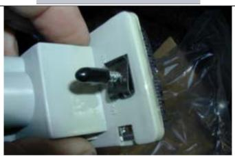
64. Remove indicators from cartons and then remove screws and speed nuts from each light. These fasteners are not to be reused – new screws are supplied in the fitting kit.
