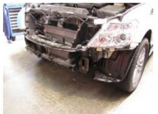
3. Remove the bumper bar from the vehicle by removing all screws and clips.
