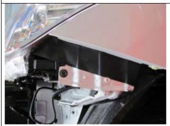
28. Place the guard cover sticker on the front lower section of each guard as shown.
