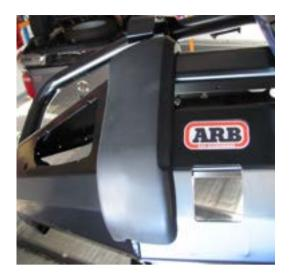
38. Fit the buffers to each side of the bar using M6 flange nuts. Torque to 4Nm max
