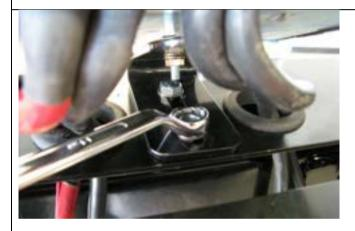
45. Using M8 fasteners fit control box mounting bracket to pan
