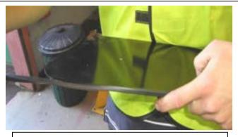
Applying trim rubber, note the join is at middle of the rear of the plate or long side.
