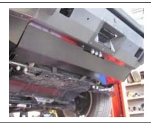
74. Fit the under panel to the bar using M6 x 20 BZ Hex screws, M6 BZ Spring washers and M6 BZ Flat washers.
