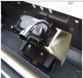
59. Carefully fit the radar sensor removed in step 11 to the bar as shown using 2 x M6 x 16 hex bolts, M6 spring washers, M6 washers and M6 flange nuts. Ensure that the sensor is level to the bar and tighten fasteners.
