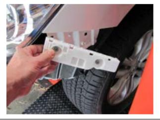
5. Remove the plastic bumper retainer blocks from each side of the vehicle and discard
