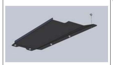
75. Fit M6 cage nuts to the under wing panels as shown.
