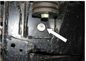
33. Place the Clevis Nuts into the holes in the side of the chassis as shown. Repeat both sides.
