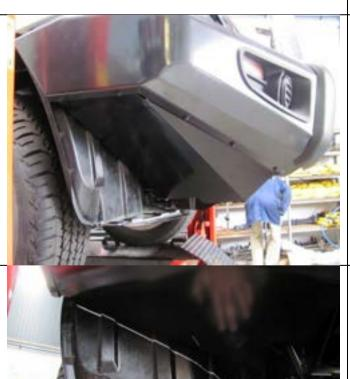
76. Fit the under wing panels to the bar as shown and attach using M6 x 20 BZ Hex screws, M6 BZ Spring washers and M6 BZ Flat washers.
