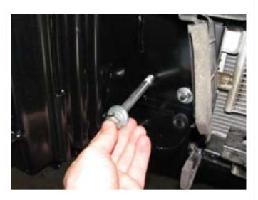
34. Place an M12 x 140 Hex Bolt, M12 Spring Washer and M12 Flat Washer (Std O.D.) through the hole in the centre of each of the Mounts into the threaded holes in the Clevis Nuts fitted in the previous step. Leave loose at this stage.
