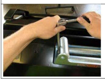
51. Fit the roller fair lead, pull only the end of the cable through and adjust the position of winch then bolt up securely. Use the 1 ½" long bolts in the top and 1 ¾"in the lower set through the RFL.
