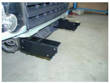
3. Fit the new impact absorbers to both the LH & RH chassis rails . **Note the profiled edge faces outward** Using the 7/16 hardware supplied , bolt the RH impact absorber into position .
