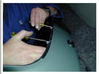
8. Placing the original bumper bar face down on a blanket remove all of the screws that hold the painted outer section to the main bumper .Using pliers remove the clip that holds the washer nozzle in the bumper and take out the nozzle (both sides). These are refitted into the bull bar once the fog lamp and turn signal are installed.
