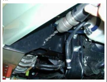
16 With assistance lift the bull bar into position and slide it over the two impact absorbers. Once in position bolt the bull bar in the 8 places using the M10 bolts & hardware supplied, finger tight only at this stage.
