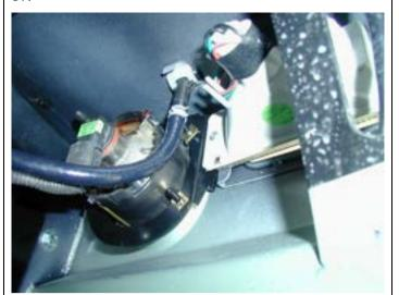
17 Re-connect the fog lamp harness on both sides of the vehicle .
