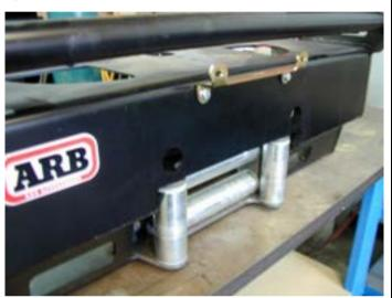
15 Attached the number plate directly to the bull bar front face using the M6 hardware supplied.
