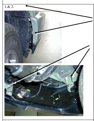
1. To remove the bumper bar from the vehicle undo the 7 screws that hold the plastic guard liner to the bumper bar on each side.
