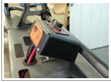
10 When fitting a winch only: Fit the control box bracket to the bull bar using the M8 x 20 mm bolts and hardware, with the open end of the bracket facing the grill. Leave these bolts finger tight at this stage.
