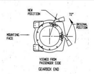
11. To place the winch clutch handle in a convenient location the winch gearbox must be rotated 2 hole spacings, 72 degrees, in an anti-clockwise direction when viewed from the gearbox end. Place the winch on its end and remove all gearbox bolts.
