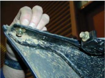
To remove the bumper bar from the vehicle, remove the 3 plastic plugs that hold the plastic guard liner to the bumper bar on each side using a small flat bladed screw driver.
