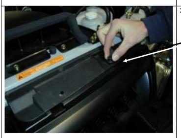
With all of the plastic plugs, two screws and two bolts removed from the lower bumper bar, the grille and grille cover must be removed. There are three plastic plugs that hold the cover in place, remove these as previously described above.
