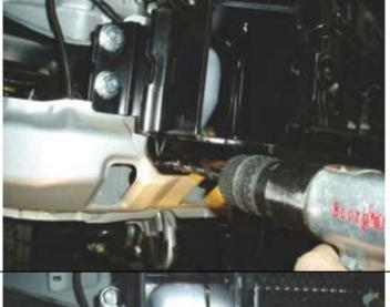
7. Drill Dia 10.5 pinning hole in lower flange of mount bracket into the vehicle crossmember
