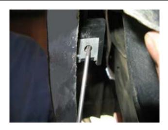
8. Remove the screws and speed nuts from the bumper on each side in the wheel arch area
