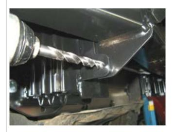
65. Using an electric drill and a 10.0 mm drill bit, drill two pinning bolt holes through the bull bar upright each side using the holes in the mount bracket flanges as a guide. One hole is located in the lower lug of the mount face and one up above the welded nuts. Use access through the light surround opening for the top hole.
