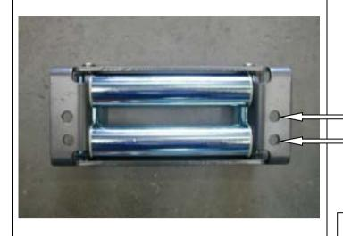
49. Using a 12mm drill bit, mark & drill two new holes in the roller fairlead 25mm below the original holes.
