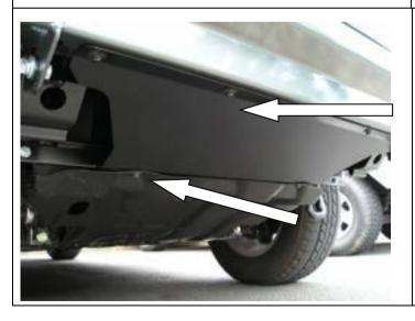
69. Attach the stone tray to the under side of the bull bar with the black M6 bolts, flat washers & spring washers.
