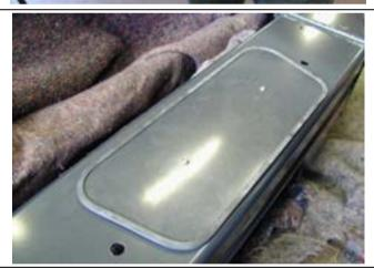
44. Fit panel to top face on bull bar using 2 x M6 dome head stainless steel screws, flange nuts and flat washers.
