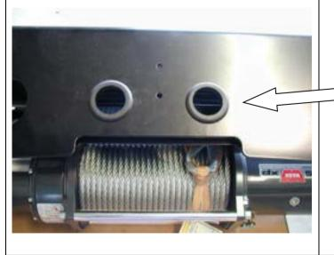
52. Insert the two rubber grommets into the top face of bull bar.
