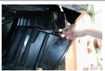
73. Trim the fender liner horizontally level with the bottom edge of the bull bar wing
