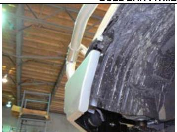
75. Push the outer edge of the liner forward past the wing return edge so that it snaps in against the wing brace as shown.
