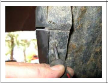
7. Remove the screws securing the fender liners to bumper in the forward wheel arch areas
