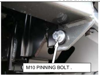
66. Fit the pinning bolts to the bull bar in the drilled positions using 4 x M10 SEMS bolt and washer sets and M10 flange nuts.
