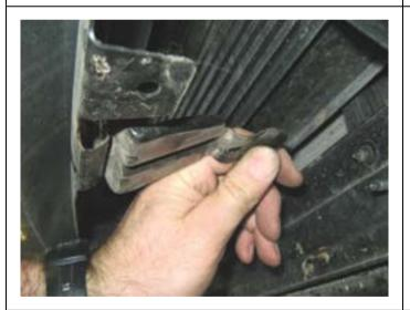
40. Bend back and up, or cut off, the leading steel support tabs on the grille support beam. These tabs previously supported the lower bumper section now removed.
