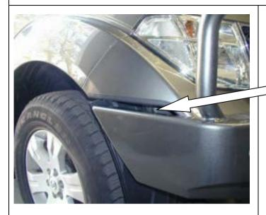
59. Ensure the bull is sitting on the vehicle level and the gap between the bumper bar and the bull bar wing is parallel.
