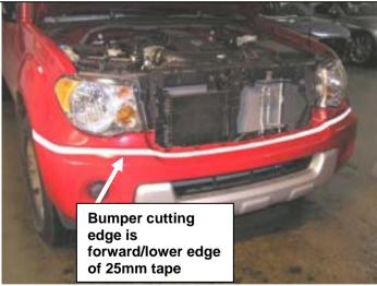
10. On bumper, apply 25 mm tape strip along low side of groove and up to corner of grille connection flange as shown
