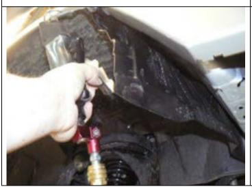
74. Trim the fender liner vertical edge so that it has about 20mm (3/4") overlap to clip in behind wing return
