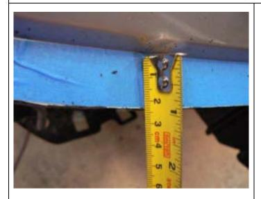
18. Using an electric jig saw with a fine to medium cutting blade – cut along the lower/forward edge of the 25mm (1") tape strip. Start the cut in the wheel arch area working from one side to the edge of the centre section to be cut by hand. Cut through both the back edge of the bumper and the plastic guard liner. An assistant at this stage could hold the bumper cover in place to ensure a straight & level cut.
