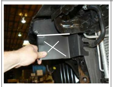
28. Trim air deflectors both sides as shown at horizontal line with a hacksaw blade or sharp cutting blade and discard the lower section as shown
