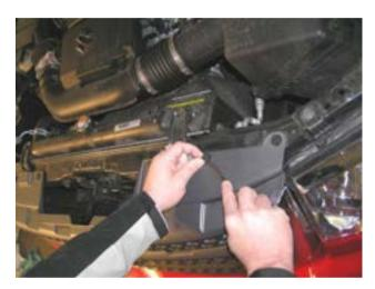
9. Remove grille by removing plastic clips in top flange, then releasing clips along lower back edge into bumper flange. Set aside.
