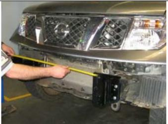
39. Check the overall width of the mount brackets by measuring the distance inside the faces as shown. The ideal width is 910mm; adjust the brackets to achieve this width, but leave hand tight
