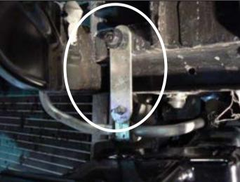
29. Remove the hanging strap supporting the power steering pipe clamp
