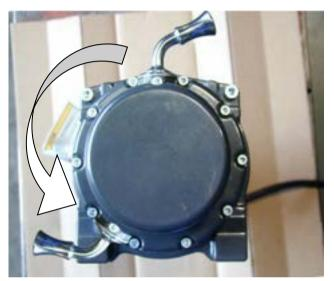
46. Remove the cap head screws retaining the gearbox to the winch drum. Carefully lift the gearbox a small amount (5 mm) and rotate144 degrees counter clockwise (four hole spacings) and re-fit the cap screws. This places the winch handle in the correct orientation.
