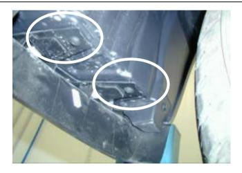
6. Remove the two bolts and screw from the fender opening area each side that attaches the bumper bar to the plastic inner guard liner as shown.
