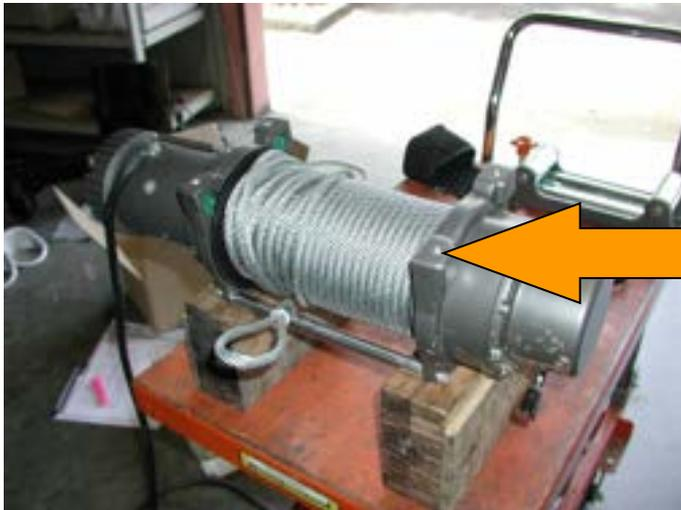
**39. To fit winch into bar you must pack winch up on a bench to enable you to lower bar down on winch, then fit four 3/8" square nuts into winch lugs.**
