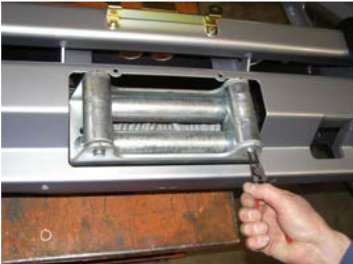
**42. Place roller fairlead over lower holes and again secure using 3/8" hardware (1 3/4" x 3/8" bolts) flat and spring washers.**
