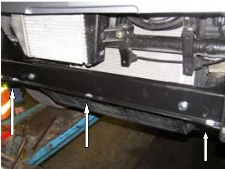
**32. When impact absorber is securely bolted to vehicle, fit 8mm caged nuts to mounting assembly.**
