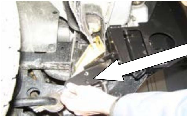
**23. Before fastening impact absorber to vehicle, fit rear brace in between impact absorber and chassis and align rear holes with vehicle chassis holes.**
