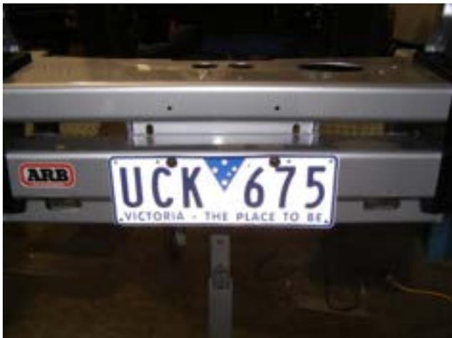
**68. If you are not having a winch fitted to the bar, fit plastic grommets into the round holes and secure using black pan head screws to secure number plate to bar as per photo.**
