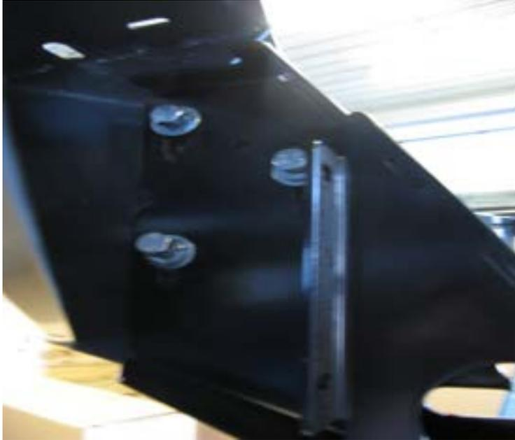
**49. With the help of a friend, lift bar in between impact mounting bracket and align slots on mounting bracket to the slots on the side of bar. Secure using M12 x 1.75 x 35 coarse pitch bolts, M12 spring, M12 flat washers and M12 flange nuts. At this stage do not over tighten the bolts to allow for bar adjustment.**
