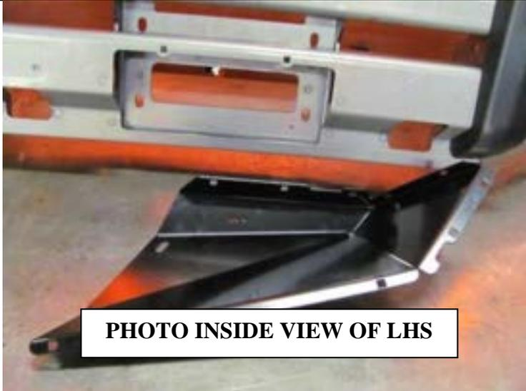
**60. Fit M6 caged nuts into both L/RHS of under wing surround panels. ( 8 per side )**
