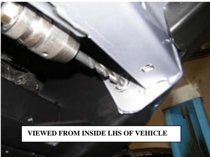
**52. When all the six bolts have been tighten firmly, using the lower holes from inside the bar as a template, drill through the impact absorber bracket using a 10mm drill bit and fasten with a 10mm SEMS bolt and a 10mm flange nut.**
