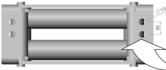
**41. Drill two new 13mm holes in the roller fairlead provided in the kit, as shown on the adjacent picture.**
