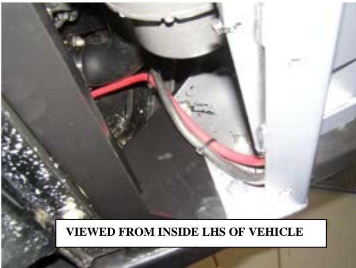
**54.** When bar is secured to mounting bracket, connect winch cables to battery and cable tie cables together to clear of all moving parts, sharp edges and hot parts.
