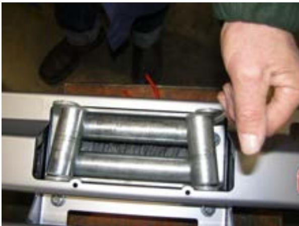
**44. Using screwdriver move vertical rollers sideways and tighten all bolts using socket and extension.**
