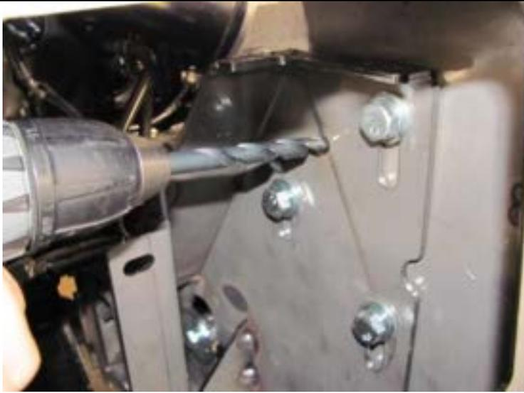
**53.** Now using the fog light opening as access drill a 10mm hole in the top of the bars upright using the hole in the impact absorbers mounting blade as a template, the pin using M10 SEMS bolt and flange nut, tighten bolt to specified torque.
