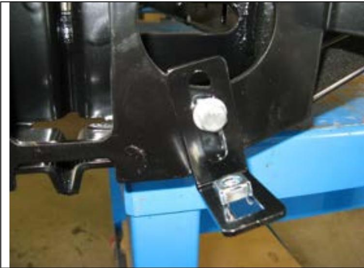
**59. At this stage loosely fit the adjustable wing under panel bracket to the mount assembly.**
