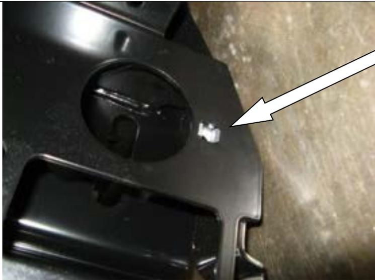
**57. The next step is to fit the wing under panels, firstly M8 cage nuts must be fit to the mount assembly as shown.**
