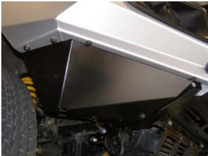
**61. Fit wing panels using black M6 hardware as per photo to both sides of vehicle. ( 4 per side )**
