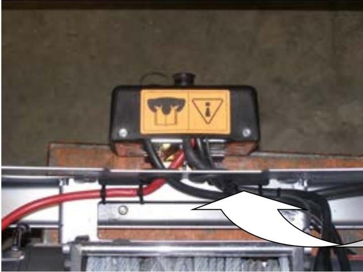
**46. Fit rubber grommets into round holes in top of bar, then fit control box to control box bracket and pass cables through rubber grommet.**
