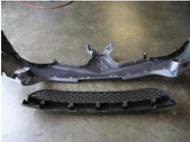
**7. With the bumper removed, you must remove lower grille section and fog light aperture rear panels, then refit bumper to vehicle.**
