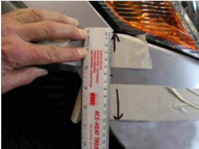
**8. At this stage draw a point 120mm down from panel line on each side of vehicle and 20mm in the centre. (AS PER PHOTO) Using masking tape, join points to points across the front of the vehicle then remove bumper from vehicle. Using a jig saw or a small hand saw, cut across drawn line. Dress up with a file.**
