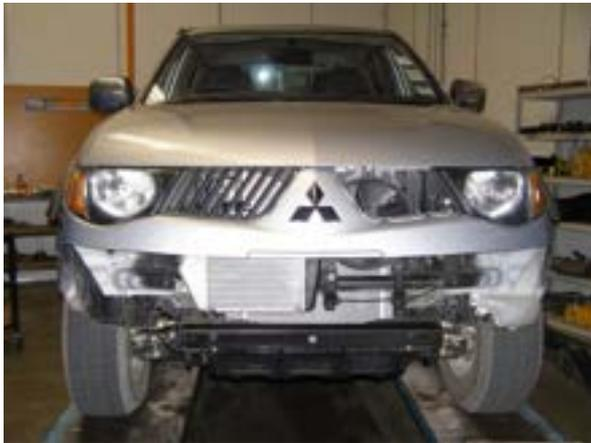
**21. At this stage the vehicle is ready to fit impact absorb mounting assembly.**
