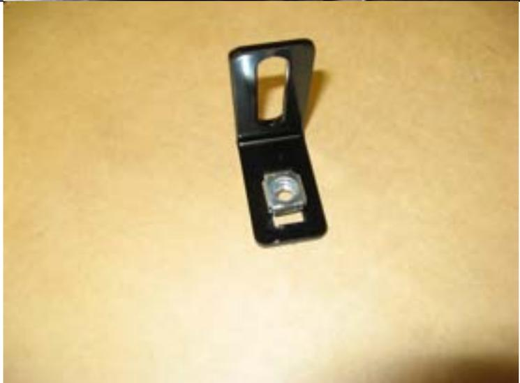
**58. Also M8 cage nuts must be fit two the adjustable wing under panel brackets as shown in the figure to the left.**
