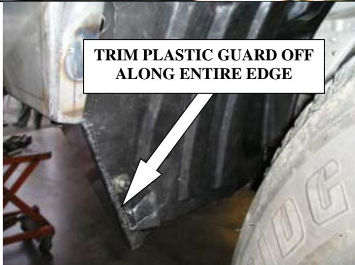
**67. Now using the edge of the wing under panel as a template trim the fender liner to suit.**
