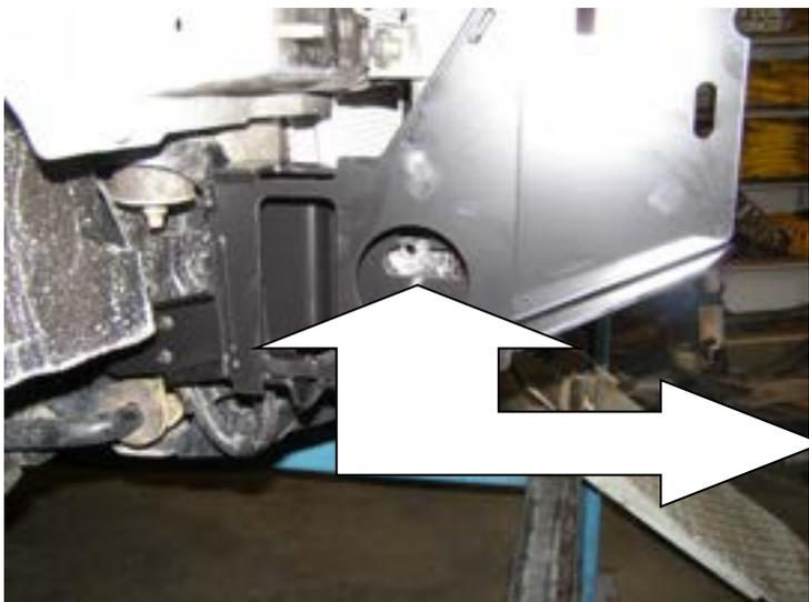
**22. Fit impact absorber mounting assembly to vehicle chassis.**
