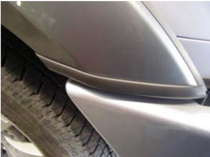
**50. Using body molding strip, fix to lower section of cut flare and trim to fit.**
