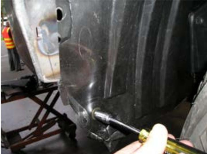
**66. Push the fender liner past the wing return and secure the fender liner mounting points using M6 hardware (4 per side).**
