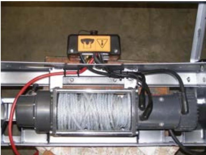
**47. Fit all 3 cables to their correct terminals and tighten. Refer to Warn installation instruction when wiring up winch. Fit plastic boots over terminals. Cable tie cables to bar as per photo to clear of all moving parts.**
