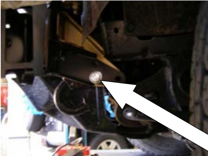
**25. LHS side has a hole only, where a 10mm x 30mm 1.5 SEMS bolt is fitted and secured by a 10mm flange nut.**
