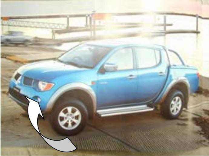
1. To fit a bar to vehicle, the plastic bumper, grill panel has to be cut.
