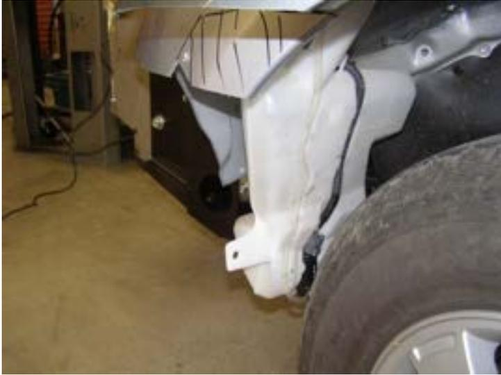
**20. When you are about to cut the LHS of vehicle, you must temporarily remove the washer bottle to enable to cut the lower section of the guard panel. Refit flare and washer bottle after cutting.**
