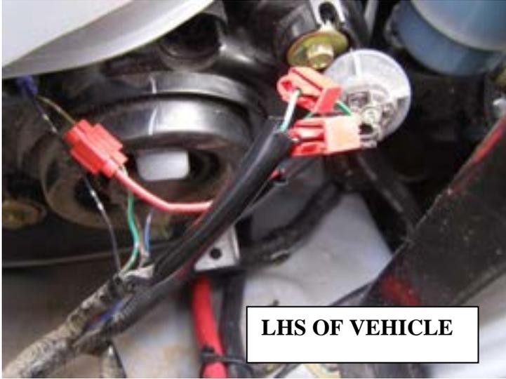
**56. Pull indicator loom up into engine bay to scotch lock wiring onto vehicle indicator/clearance lamps**
