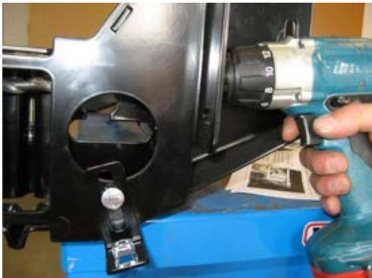
**30. Using a long 10mm drill bit, drill through vehicle body mount using hole in mount as a template, secure using 10mm X 30mm SEMS bolt, 10mm flange nut. When both sides of vehicle are done, tighten firmly.**
