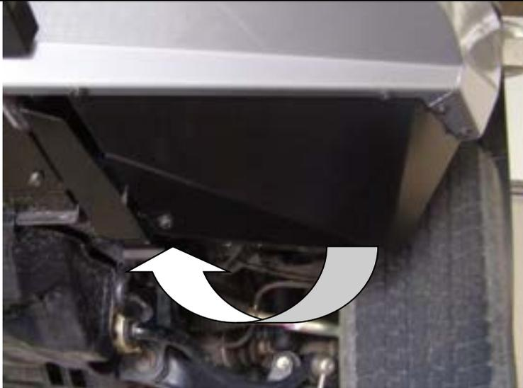
**62. Now position the adjustable wing under panel bracket so that it aligns with the lower slot on the wing under panel and tighten the bracket in place.**
