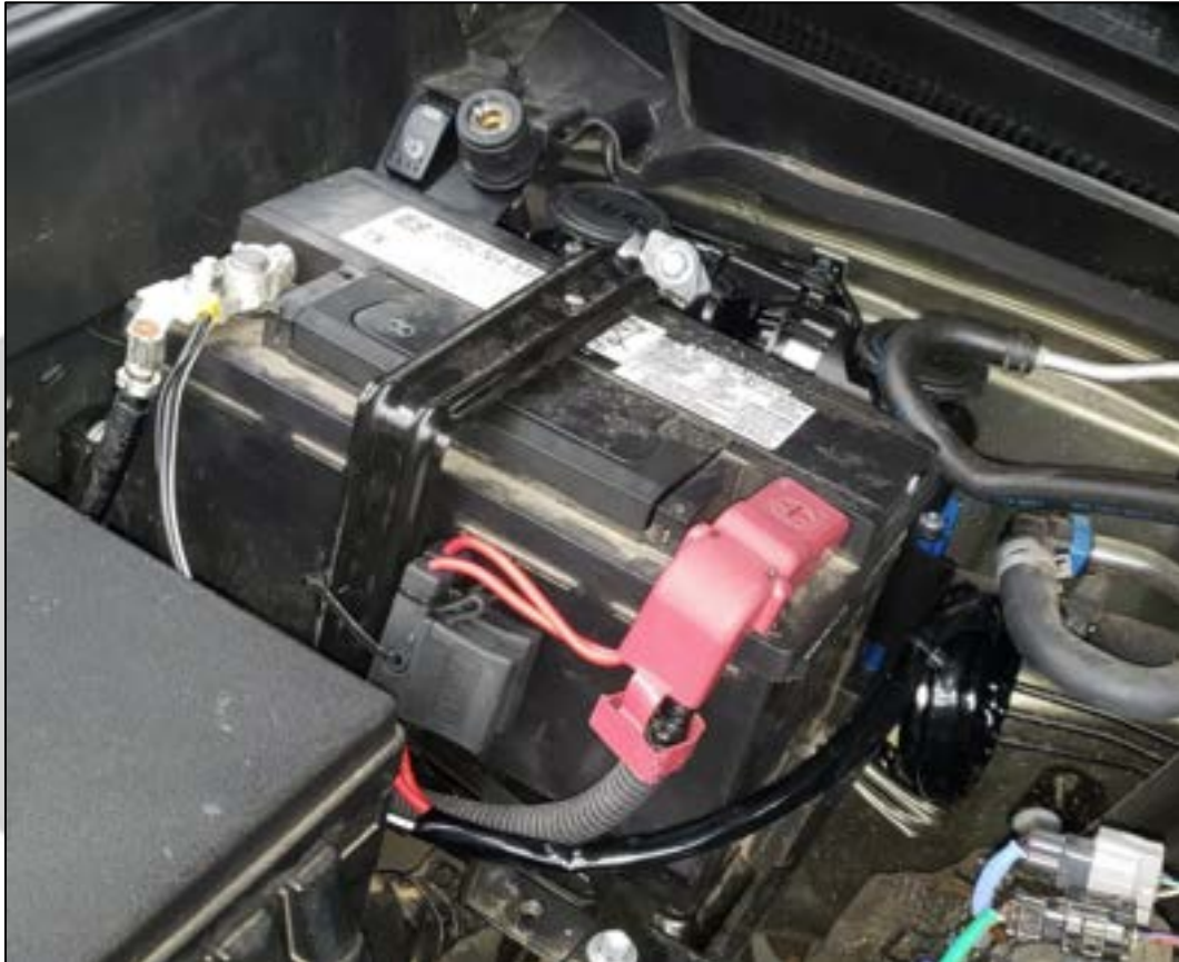
Figure 19. Brushed Compressor harness fuse location
