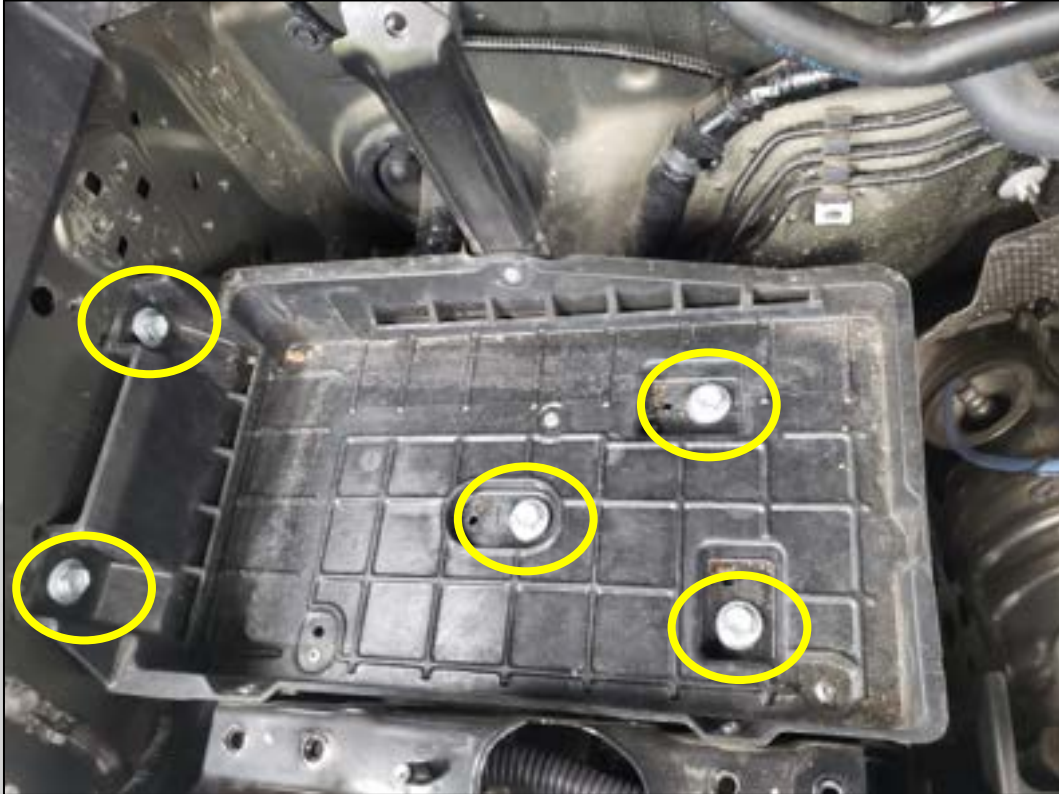
Figure 13. Battery tray and original fasteners
