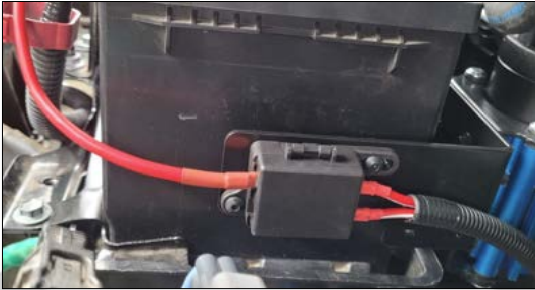
Figure 20. Brushless Compressor harness fuse location
