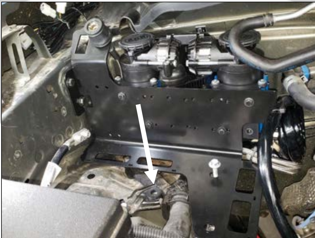
Figure 17. Compressor bracket assembly spacer washer
