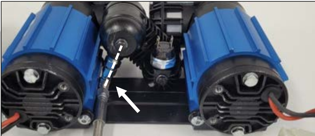
Figure 7. Positioning of the reinforced air line by manifold cap rotation
