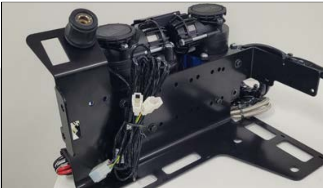
Figure 9. Compressor bracket assembly ready for installation into a vehicle
