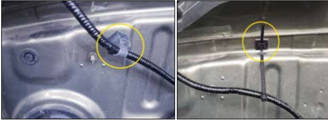
Figure 16. Original cable retainer and replacement adhesive cable tie retainer
