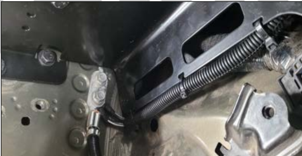
Figure 21. Preferred body grounding point
