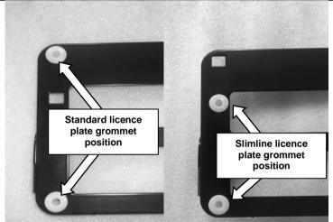
Insert 4 plastic grommets into number plate frame to suit licence plate size
