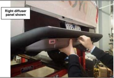
38. Position the diffuser panels on either side of the receiver tube as shown.
