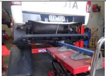
With the assistance of other people or a lifting device, lift the RSTB up beneath the chassis rails aligning the threaded holes in the side of the chassis with those in the vertical surfaces of the RSTB.
