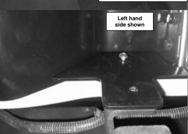
36. Fit infill plate on either side of licence plate as shown using 1 M6 X 16 Stainless button head screw per infill plate. Only hand tighten fastener at this stage ensuring second hole is aligned.
