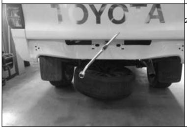
2. If required remove the spare wheel from beneath the tub using the wheel nut wrench and jack handle pieces supplied with the vehicle. Insert as shown through the access slot above the number plate position and rotate counter-clockwise to release the wheel.
