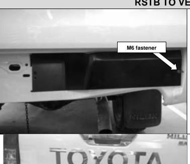
18. Attach beaver panel to rear of tub as shown using single M6 fastener
