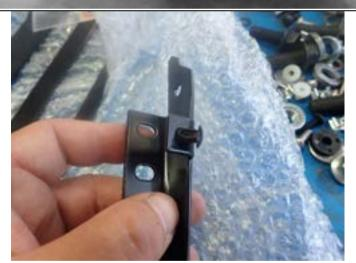
21. Insert canoe clip into both LH and RH number plate mount brackets as shown.
