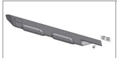
37. Fit the diffuser mount plate with an M6 x 16 M6 Stainless Steel button head screw and M6 flat washer to either the LH or RH diffuser as shown.
