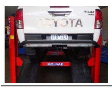
41. Attach the step plate extrusion to the RSTB using 8 M6x1.0x16 button head screws. Proceed to tighten fasteners installed in step 61
