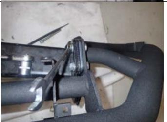
When tighten bolts, tighten them sequentially, alternate between LH and RH sides.
