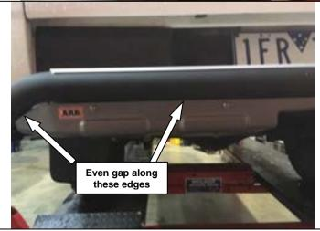
40. Position each diffuser panel so there is an even gap between the panel and the RSTB tube. Tighten fasteners to the specified torque.
