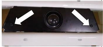
Fit the panel over the radar sensor and attach to the panel brackets using 2 x M6 button head cap screws.
