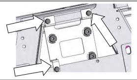
5. Attach the bracket to the bar from the rear as shown using M6 x 20 hex bolts, spring washers, flat washers and flange nuts.
