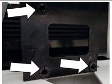
Take the plastic clips from step 3. Push them 6. into the 3 holes in the new radar mount from the front of the bull bar.
