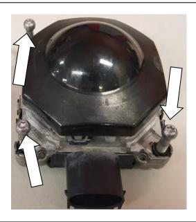
Remove the 3 Torx drive ball screws from the radar and refit from the back side .Leave approx. 3 turns of thread visible on the screw. **Do not** bottoming out the bolt into the plastic thread.
