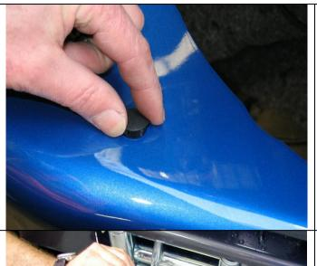
Unless fitting CB aerials, fit blanking plugs in provided holes in the top of the wings. 80.
