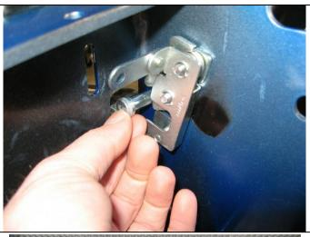
62. Fit the striker pin to the *RHS* hinge plate and secure with 5/16"UNC nut and spring washer as shown and tighten to 22Nm or 16lbft
