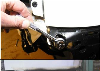
21. Remove bumper cover retaining brackets from the fenders.
