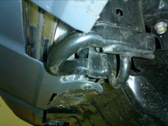
2. Remove tow hooks and bolts, set aside to be refitted.
