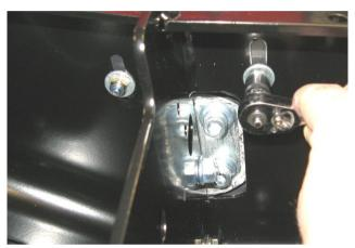
59. Slide the buffers down over the frame and secure using M6 flange nuts on the four lower buffer studs on each buffer and M6 nyloc nuts with large M6 flat washers on the two studs located on top face.
