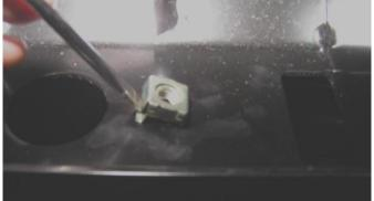
53. In lower inside face of pan, fit M8 cage nuts for stone tray in four positions as shown.
