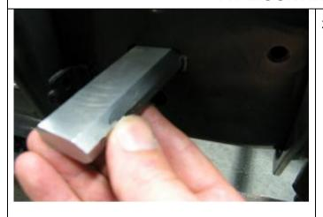
23. Insert clevis nut into rectangular hole in the inboard face of chassis, ensuring the threaded end is inserted first.
