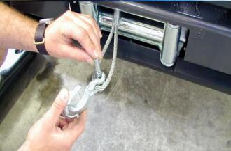
81. If winch fitted, fit off winch hook.
