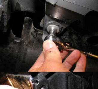
3. Remove lower bumper retaining screws.
