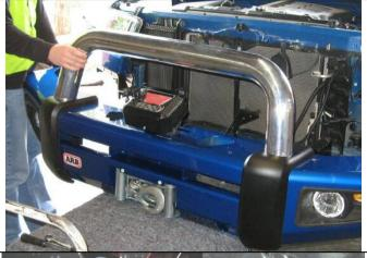
75. Using two people, three if winch fitted, position the bar assembly on the vehicle mounts.
