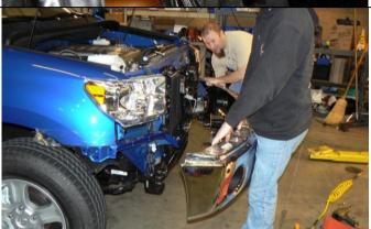
Remove crash bar and lower bumper assembly and set aside, retain flange nuts for reuse.
