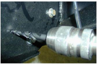
64. Using the M10 pilot hole in mount brackets, drill pinning hole through uprights of bull bar. Fit M10 SEMS bolt and flange nut, do up tight to recommended torque.
