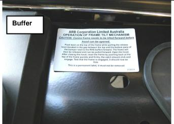
83. Apply the frame tilt operation label to the top face of the pan adjacent to the buffer as shown in diagram
