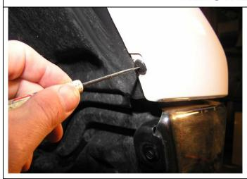
5. Remove upper fender liner retaining scrivets.
