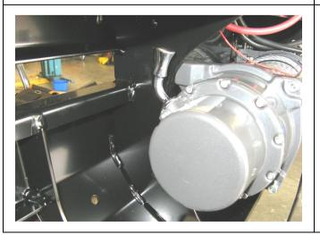
36. Position the winch with the mount face facing upward on an adjustable table or similar and with the assistance of another person lower the bulbar over the winch. The winch handle should be in the LHS of the bull bar for smaller winches than 12-15000lb winches which are on the opposite side as they spool in the opposite direction. The cable must always spool off the bottom of the winch.
