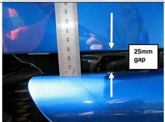
80. Adjust the bar height leaving approximately 25mm gap between top of wing to fender. Align the bar so the front face is vertical and the gap is even on both sides of the vehicle.
