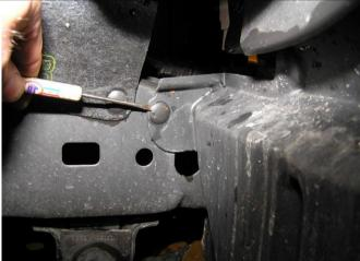
6. Prise out lower fender liner plastic push in plugs. Remove lower fender liner completely, they will not be reused.
