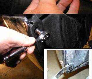
4. Remove all lower fender liner retaining screws to bumper.
