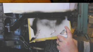
22. Mask up and spray paint the exposed metal trim area black satin, from the wheel arch right around to the inboard headlamp area as shown, both sides of the vehicle.
