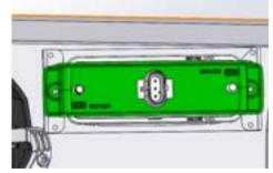
13. Install LED lamp with bracket into bull-bar using 2 x 15mm mounting screws provided. (RH Shown).
