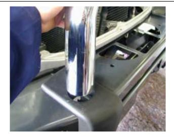
15. Push the top Sahara tube through the hole in the buffer and fasten using the M12 x 40mm bolts, washers and spring washers.
