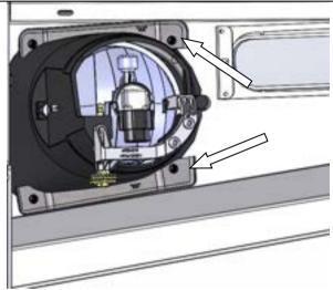
11. Secure into position as indicated using the 2 x fog lamp clamps and 4 x self-tapping screws.
