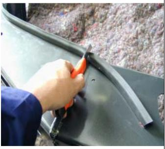
34. Using a sharp knife cut the excess rubber in line with the inside end of the wing. Only cut the inside excess, the other end will be cut when the winch bumper is fitted.
