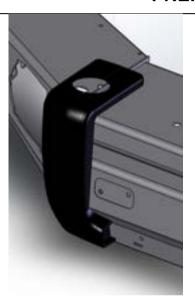
8. Insert the side buffers through the holes and fix using the M6 flange nuts. (Do not over tighten). (RH shown).
