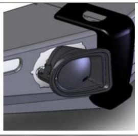
10. Fit fog lamp housings (3163082) into the bull-bar fog lamp cutouts as shown. (RH Shown).
