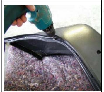
33. Using a Phillips head screw driver or cordless drill with a Phillips head tip fix the extrusions to the top of the wings using the self-tapping screws.
