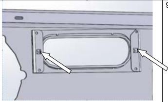
9. Install Nylon plugs (6821116). (4 off) Into Clearance Light/Turn Signal Brackets. (RH Shown).
