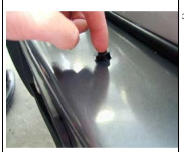
39. There are two 16mm dia. holes located on the top face of the bar. If no CB aerials are to be fitted the holes can be covered with the plastic plugs provided in the fitting kit.
