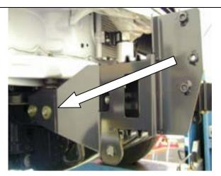
Mount the Impact Absorber brackets to each side of the chassis using original fasteners.
