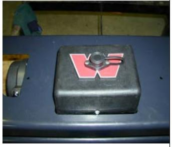
24. Fasten control box assembly to the bar using the M6 x 16mm bolts and flange nuts.
