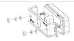
12. Install 6821285 bracket onto LED lamp with 2 x flat washer, 2 x spring washers and 2 x M6 nuts as shown.
