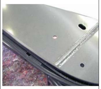
32. Insert the mount strips inside the channel section of the rubber extrusion. Make sure the flap section is on the outer side. Allow generous even amounts of excess at either end of the strip so that it can be trimmed later.
