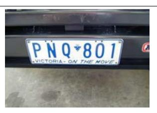
19. Bolt the number plate through the top holes using M6 X 16mm bolts and M6 flange nuts. If desired double sided tape can be used down the sides of the number plate.
