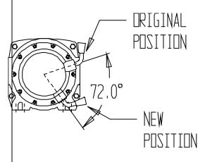
20. To place the winch clutch handle in a convenient location the winch gearbox must be rotated 2 hole spacing's, 72 degrees, in a clockwise direction when viewed from the gearbox end. Place the winch on its end and remove all gearbox bolts. Gently raise the gearbox just enough to rotate it. Do not completely remove the gearbox and avoid damaging the gasket. Refit all bolts and tighten.
