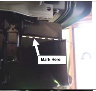
30. Mark the lower section of the air scoop for the power steering radiator as shown. This is for trimming to clear the mount brackets.
