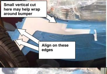
11. Ensure template is correctly positioned along the edge of the bumper both at the front quarter panel as well as along the wheel arch. Mark along cut edge with a marker.
