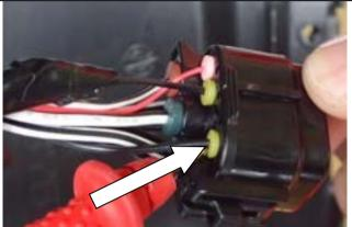
75. If installing driving lights, the high beam signal can be tapped into on the passenger side of the vehicle using the black wire on the black plug shown.
