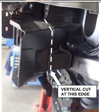
Mark out a vertical cut line on the 34. LHS air deflector.
