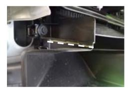
31. Now mark along the lower bend as shown, now cut the shroud along the marked edges as shown
