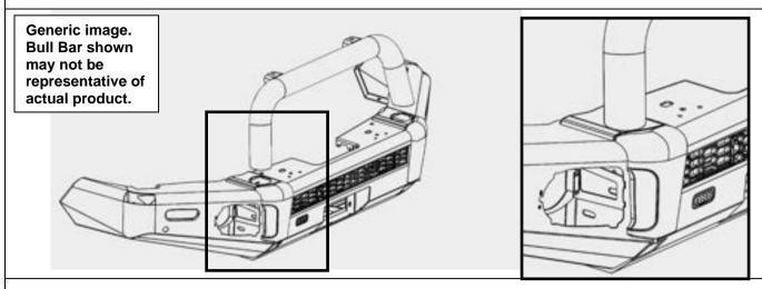
58. Fasten top tube to the bar using 4 x M10 SEMS Bolts. Adjust position of top tube left/right until it sits central on the bar and the rear buffers are positioned correctly. Tighten M10 SEMS Bolts to specification. Tighten Rear buffer screws.
