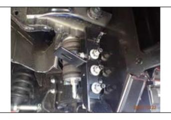
96. Fit both wing panel brackets to the higher holes in the outside of the mounting brackets using M8 bolt, washer and flange nut.
