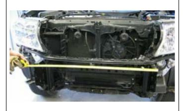
67. Tap the outer flange of the mount brackets until they are hard up against the tow hook mount area. Nip up the lowest outboard nut on each bracket. Brackets should be less than 935mm apart.
