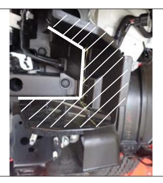
35. Mark out a second line to meet up with the line in the previous step. Cut the air deflector on the LHS of the vehicle using a multi tool or similar. Shaded area shown must be removed.
