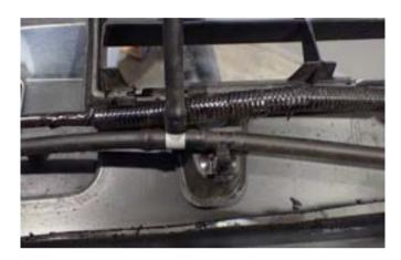
23. Remove OEM Fog lights, Parking sensors, washer lines and electrical loom from bumper, these will be reused. Label which side parking sensors are taken from for refitment.
