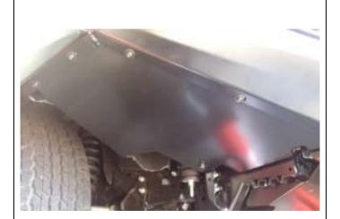
99. Trim the fender liner end flush with the splash panel face as shown. Then tuck the remaining wheel liner inside the wing panel return.
