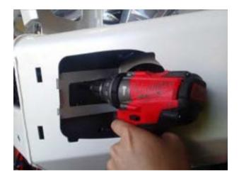
89. Using the M10 pilot holes in the bull bar uprights, drill the two pinning holes through mounting brackets on each side. Fit M10 bolt and washer sets and flange nuts and tighten to specified torque.
