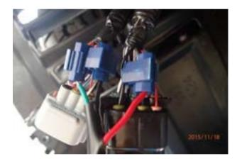
**CONNECTING LED INDICATOR/CLEARANCE (PASSENGER SIDE)**
