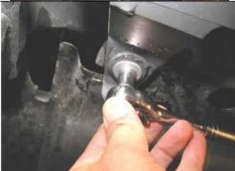
5. Remove lower bumper retaining screws.
