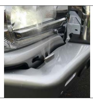
88. Check HLW Function; ensure there is adequate clearance between bull bar and extended HLW units.
