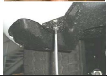
Remove lower trim panel sets each side which attach to bumper and engine protective plate area then set aside, they will not be reused.
