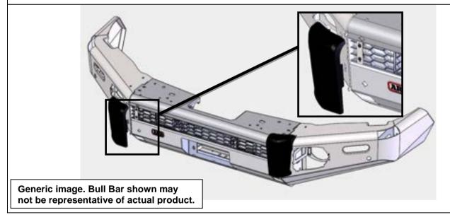
54. Ensure each buffer sits flat against the face of bar. Secure wing side using retaining clips. Secure inner side using the angled cup washers, flat washers and screws.
