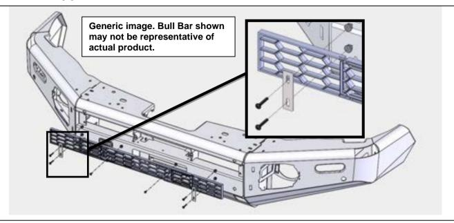
53. Place each of the front buffer sections onto the bar as shown. Ensure that the 2 lugs and 2 screw bosses pass through the holes in the bar.
