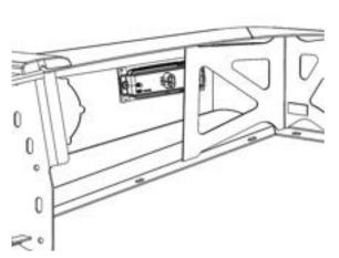
60. Fit the small plastic grommets to the bar and attach the combination LED lamps to the bar using the screws provided with the lamp kit. Details provided in Fitting instruction 3789197.
