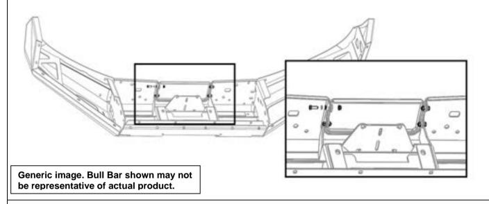
44. Fit the number plate bracket to the top face of the lower-centre pan on the bar using 3 x M6 x 20 hex bolts, flat washers and flange nuts.
