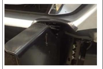
69. Fit pinch weld to the cut edge of the bumper as shown.
