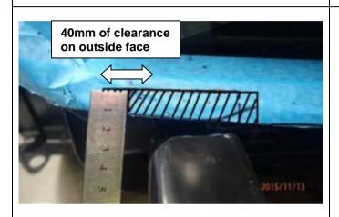
68. The Mounting brackets will contact the bumper, mark a rectangular cut on the bumper to ensure that there is a minimum of 25mm of clearance between the mounting bracket and the bumper. 40mm clearance is required on the outside face of the mount. Remove shaded area of bumper.
