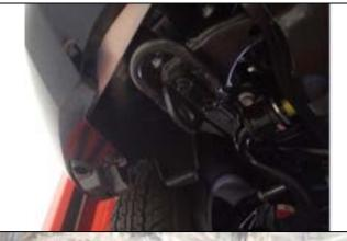
9. Remove right and left splash guards located at the recovery hooks.
