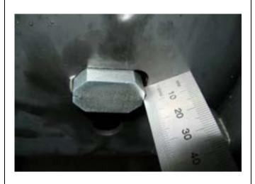
85. Then tighten up the long M12 chassis studs, ensuring that the clevis nut is positioned correctly over the hole in the chassis.
