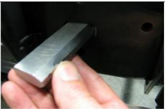
61. Insert clevis nut into rectangular hole in the inboard face of chassis, ensuring the threaded end is inserted first.
