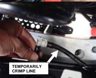
19. Unplug head light washer fluid line. Crimp line to prevent washer fluid draining out with brake line clamp.
