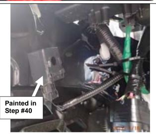
76. Once satisfied that sturdy electrical connections have been made on both sides, cable tie both harnesses back onto the sheet metal underneath the headlights as shown.
