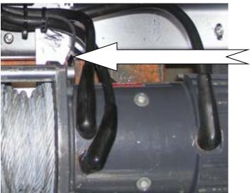
47.Fit ground wire under winch tie rod. ( See Photo )
