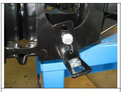
67.At this stage loosely fit the adjustable wing under panel bracket to the mount assembly.
