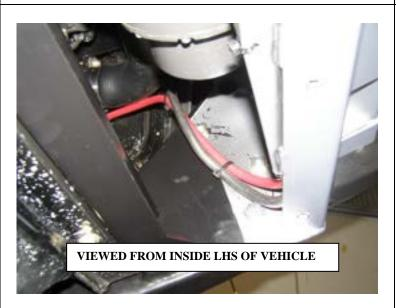
54. When bar is secured to mounting bracket, connect winch cables to battery and cable tie cables together to clear of all moving parts, sharp edges and hot parts.
