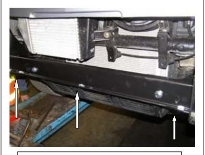
31. When impact absorber is securely bolted to vehicle, fit 8mm caged nuts to mounting assembly.
