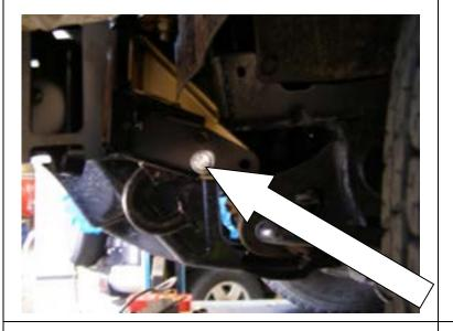
24.LHS side has a hole only, where a 10mm x 30mm 1.5 SEMS bolt is fitted and secured by a 10mm flange nut.
