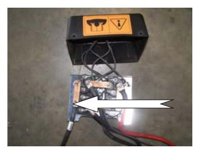
37.To fit control box to bar, you must change the arrowed lead (yellow tagged) in photo with the longer lead that is supplied in fitting kit. When all is fitted, screw plastic cover back onto control box.
