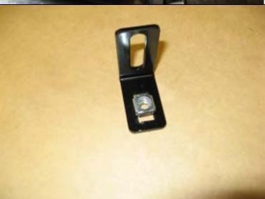
66.Also M8 cage nuts must be fit two the adjustable wing under panel brackets as shown in the figure to the left.
