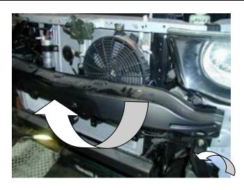
6. Remove cross member and mounting brackets from vehicle.
