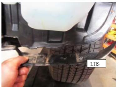
72.Remove plastic inner guards and cut off lower flange as shown.
