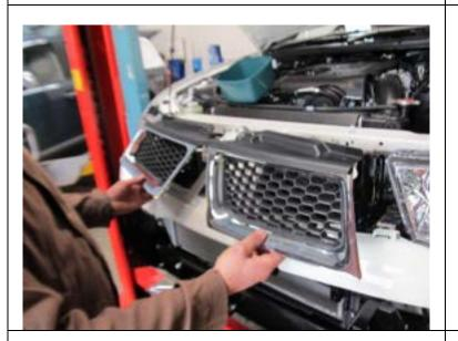
7. Remove the two Grill Panels first, to access Bumper retainers.
