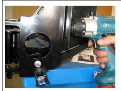
29. Using a long 10mm drill bit, drill through vehicle body mount using hole in mount as a template, secure using 10mm X 30mm SEMS bolt,10mm flange nut. When both sides of vehicle are done, tighten firmly.
