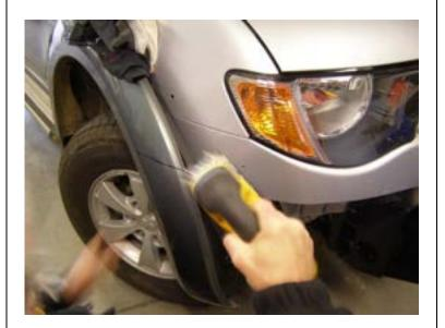
14. Lift flare away from vehicle, and cut along the drawn line, follow the same procedure on the other side.
