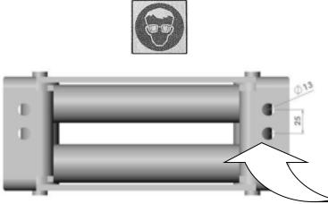
40.Drill two new 13mm holes in the roller fairlead provided in the kit, as shown on the adjacent picture.
