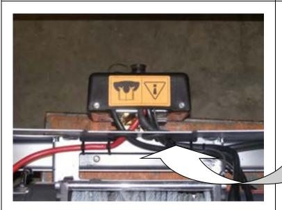
45. Fit rubber grommets into round holes in top of bar, then fit control box to control box bracket and pass cables through rubber grommet.
