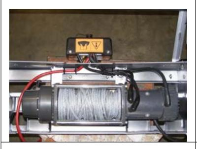
46.Fit all 3 cables to their correct terminals and tighten. Refer to Warn installation instruction when wiring up winch. Fit plastic boots over terminals. Cable tie cables to bar as per photo to clear of all moving parts.
