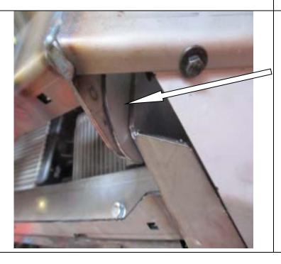
48.Before fitting the Bar, tape Packer Plates to the inside face of Chassis Mount (One per side at this stage).
