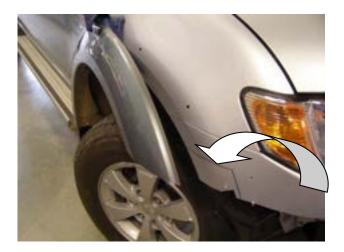
18. Once again lift flare away from guard and cut out marked section.
