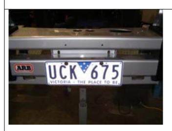
78.If you are not having a winch fitted to the bar, fit plastic grommets into the square holes and secure using black pan head screws to secure number plate to bar as per photo
