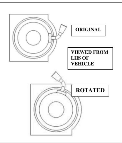
TO FIT A WINCH BAR 36.To fit an 8/9/9.5/000lb winch, rotate gearbox 72° counter clockwise.
