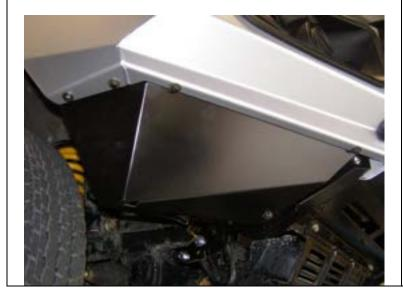
69. Fit wing panels using black M6 hardware as per photo to both sides of vehicle. (4 per side)
