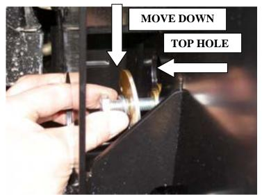
25.Using M10 x 50 x 1.25 mm bolt, 10mm spring washer, large flat washer and packer, feed into top hole and move down and screw bolt into captive nut in chassis.
