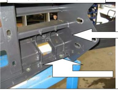
32. The next step is to fit the buffers to the bar using 6mm flange nuts, 6 per side. ( DO NOT OVER TIGHTEN )
