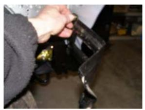
5. Remove flare/bumper bracket from vehicle.
