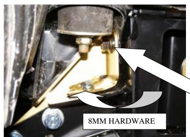
30.Lastly, fit M8 x 20mm bolt, spring washer, flat washer and 8mm flange nut to mounting assembly and tighten firmly.
