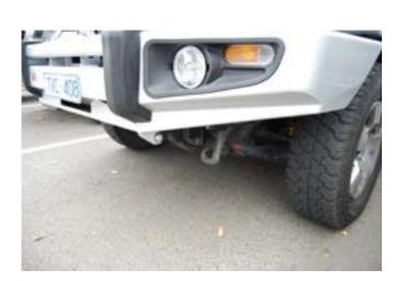
57.If optional fog lights are going to be fitted to bar, follow fitting instructions from fog light kit part no. 6821201 and wiring harness part.no.MD02
