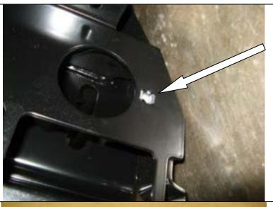
65. The next step is to fit the wing under panels, firstly M8 cage nuts must be fit to the mount assembly as shown.
