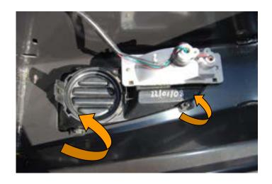
56.Install the turn signal into the rear of light insert using 2 self tapping screws 6 x 25mm pan head) supplied with the light insert fitting kit.
