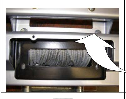
39.Lower bar down over winch, line up top holes first and secure using 3/8" hardware (1 ½"" x 3/8"bolts) flat and spring washers. (finger tighten only)
