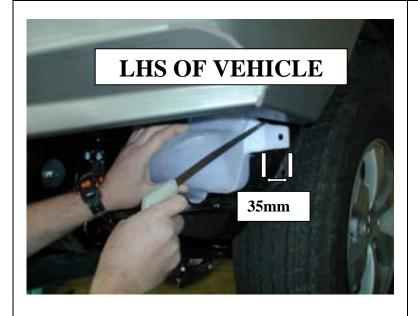
59.Before fitting under wing surround panels to bar, you must cut back washer bottle to give clearance of panel.
