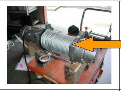
38.To fit winch into bar you must pack winch up on a bench to enable you to lower bar down on winch, then fit four 3/8 " square nuts into winch lugs.
