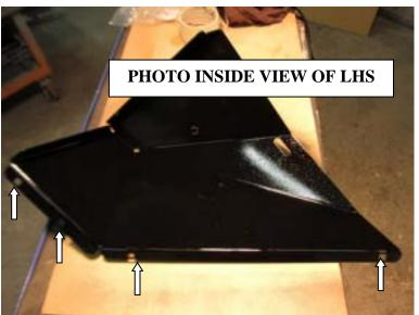
68.Fit M6 caged nuts into both L/RHS of under wing surround panels.
