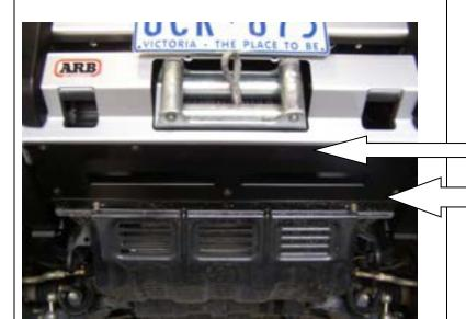
75. Fit air deflector under centre of bar using M6 black hardware at the front of bar and M8 hardware at the rear of bar.
