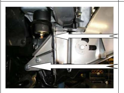
26. With the side and rear bolts fitted, fit the most rearward bolts to each side of the vehicle. Tighten all six bolts firmly.
