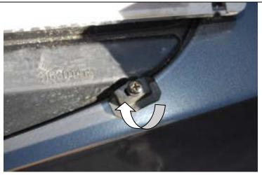
55.Fit light insert into rear of bar using 4 screws, rubber washers and retainer clips.
