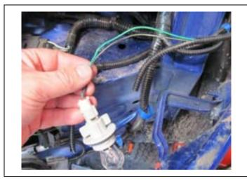
31. On each side of the vehicle, carefully cut back the protective tubing from the turn light globes wiring being careful not to damage the wires inside.
