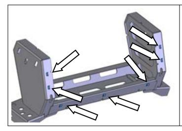
80. Fit seven M8 cage nuts into the mount bracket from the inside.
