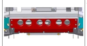
112. Attach the centre stone shield to the mount bracket using seven M8 hex bolts, seven M8 spring washers and seven M8 flat washers into the cage nuts fitted in step 80.
