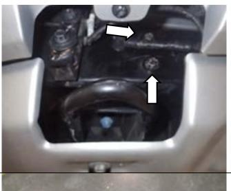
6. Supporting the Bumper, undo and remove 2 fasteners per side and carefully remove the bumper. These fasteners are to be kept and reused.
