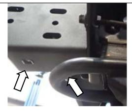
17. Install 4 x M8 cage nuts inside chassis mount.
