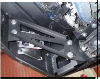
30. Install wing braces using 4 x M12x25 bolts, 4 x M12 washers and 4 x M12 nuts per side.
