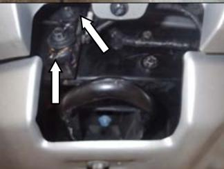
4. Remove the 2 outside fasteners from each side of the bumper mounts. These fasteners are to be kept and reused.
