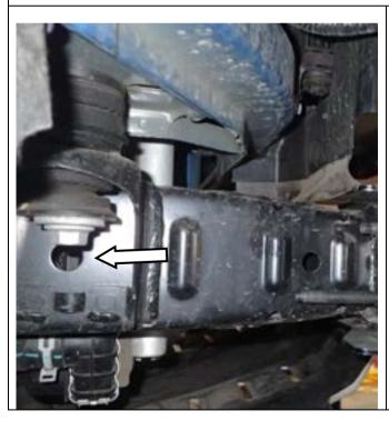
5. Using a blunt object, push the retaining clips for the Factory air scoop to loosen.
