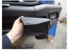
34. Fit the number plate using 2 x M6 button head cap screws, 2 x M6 washers and 2 x M6 flange nuts.
