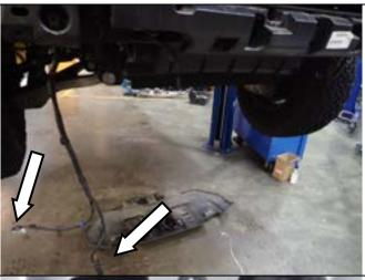
3. Disconnect the Bumper wiring loom, 2 x connectors.
