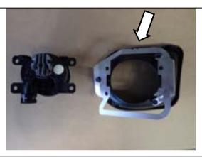
24. Fit Fog Light brackets to Fog Light housing. Take note of the 2 notches in bracket for direction, this is UP.
