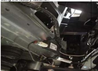
13. Using the retaining clips, fit the antenna up onto the plastic above
