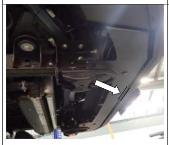
36. Using the M8x25 bolts and M8 flat washers, fit the undertray to the chassis mount. Align keeping minimum of 5mm clearance.
