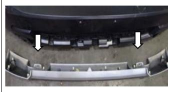
2. Remove the 2x screws used to secure the lower plastic front bar. Carefully detach piece from vehicle and set aside.
