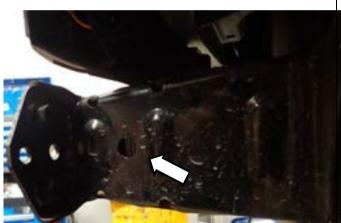
14. Insert crush tube through chassis being careful not to drop, access is attained through the front if needed.
