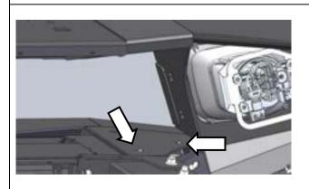
26. Fit 2 x M6 Cage nuts per side in locations shown. These cage nuts are for 3.6-4.5 thickness material. (4 off included ONLY in the Fitting kit)
