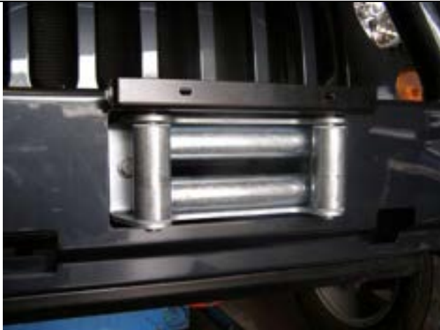
Roller Fairlead installed
