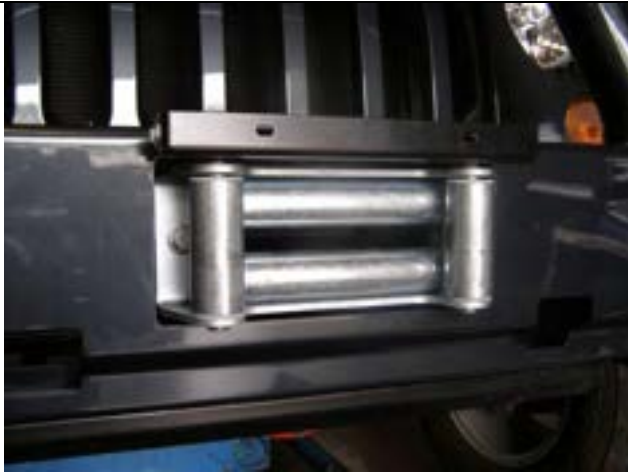
Roller Fairlead installed
