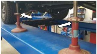
8. Place the RHS Step against the chassis Use adjustable axle stands or a second person to hold the rails in place.
