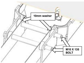
At the front mount use the M10x135 bolts and 10mm thick washers. Insert the washer as the bolt is passed through the cross member
