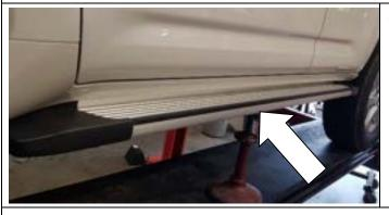
If fitted, remove the factory side steps.
