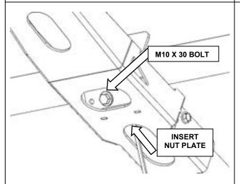
Attach the front mount to the chassis at the side using an M10 x 30 bolt and M10 nut plate.
