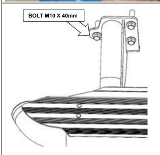
Assemble M10x40 bolts through rear step mount and into the factory chassis threads (6151717).
