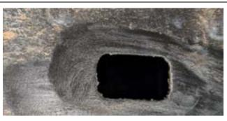
10. On the chassis in line with the middle rail mount, remove the plastic plug to expose the hole.
