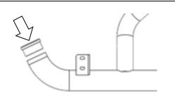
Fit the Rubber Plugs into the ends of the Side Steps.
