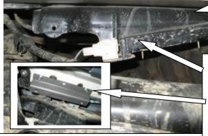
4. Remove this bracket from vehicle (shown with arrow) and relocate with new bracket supplied in kit. Make sure all wires are clear of the exhaust. Relocation bracket fitted to vehicle shown inset.
