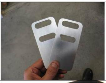
18. Make sure the distance is no less than 10mm. If not add the 3mm packers to achieve a minimum 10mm. NOTE: Distance between plastic bumper and bar must be 10mm or greater to allow for movement.
