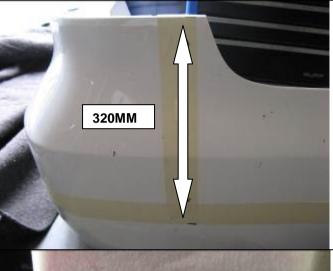
6. From the top edge of the bar measure straight down 320mm and mark. Join marked lines with a length of masking tape making sure it is straight. This will be the cut line. NOTE: Make sure line is straight by sighting down length of bumper. If not re-adjust tape so a straight line is achieved particularly around corner near reflector.
