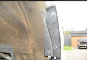
23. Cut top of original mud flap as shown and attach to vehicle and bumper with original hardware.
