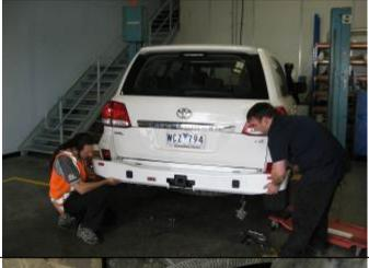
15. With the help of another person place bar gently on vehicle and secure loosely with original tie down bolts in chassis.
