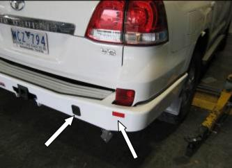
22. Install reflectors and high lift jack plugs.
