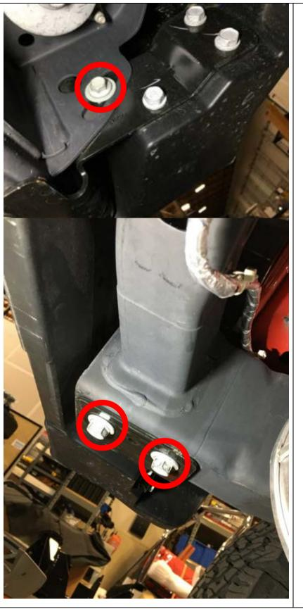
1. Start by removing the bumper. There will be three bolts per side, two on the bottom side of each frame rail and one on the rear body mount.
