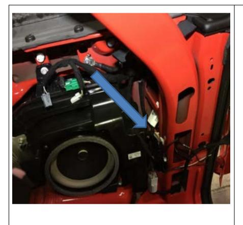
37. Unplug the large black connector and locate the dark blue wire with white trace. Splice the white wire from the extension loom onto this wire. The earth is the black wire with grey trace. Use solder and heat shrink. Secure wiring with cable ties.
