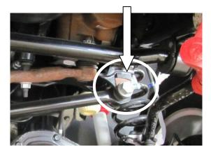
Replace with new OME Panhard Bracket re-using the OE bolts, loosely start all 5 bolts first then tighten.
