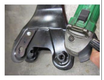
24. Nut is held on by small spot welds on the outer flanges. Grinding the edges slightly and a gentle tap with the hammer will break off these welds, do not damage arm as these are required for reassembly.
