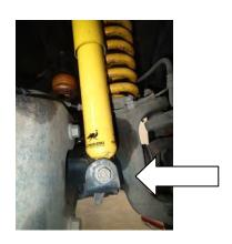
2. Where radius arm mounts to axle, loosen but <u>do not</u> remove the two M18 bolts on both Left and Right Radius Arms.
