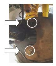
20. Lever radius arm into fixed chassis mount, using M18 bolt to fix, you may need to push/pull the wheel to get the holes to align the fastener with the mount hole.
