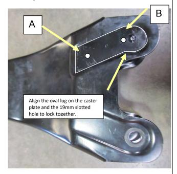
12. Fit M8 bolt (6151021), nut (6151032) and washers (4581081) to new holes drilled at ( A ) and tighten to 20 Nm.
