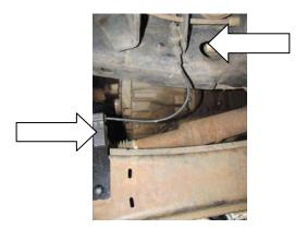
4. CAUTION: The radius arms keep the axle in place underneath the vehicle, at all times at least one of two radius arms must be fully connected. Work only on one side at a time from this step on, failure to do so may event in serious injury.
