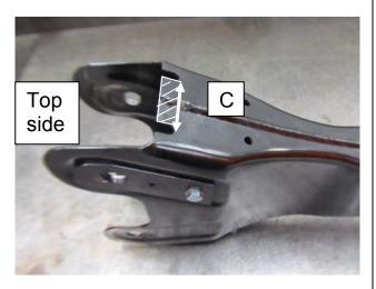
17. With finished assembly, remove all burrs making sure that castor plates are still firmly sandwiched together. If not, disassemble clean and de-burr, then reassemble unit.
