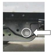
Right hand radius arm should now be secured back in place with all M18 bolts and nut threads tightened and then backed off one turn to allow ease of working on left hand side.
