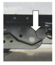
6. Remove top M18 bolt of radius arm on axle end pivot radius arm to the ground, then remove lower bolt. Arm should now be free to remove.
