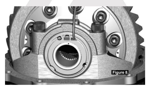
Rotate the seal housing until the square cutout lines up with the locking tab position at the center of the bearing cap. (Fig.8.)
