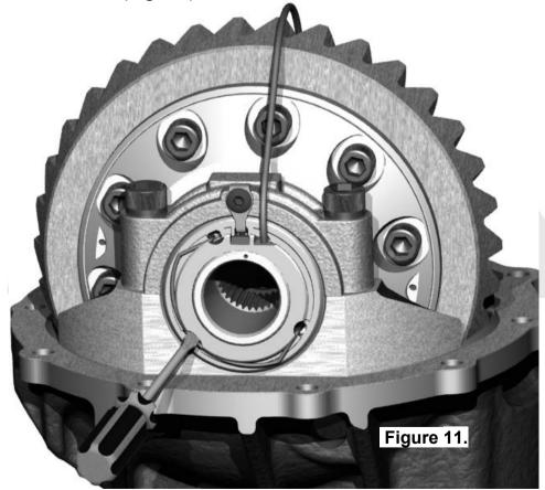
☐ Check that the seal housing is now secured from rotating and that it is still sitting flat against the adjuster nut.
