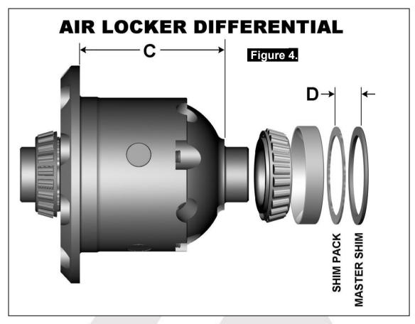
Measure the distance from the Air Locker bearing shoulder to the ring gear mounting face (shown as 'C' in Fig.4.) and record this measurement as 'C'.
