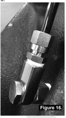
☐ Push the airline into the compression fitting body and screw the outer nut down onto it. Using a 12mm spanner, tighten the outer nut onto the compression fitting body.
