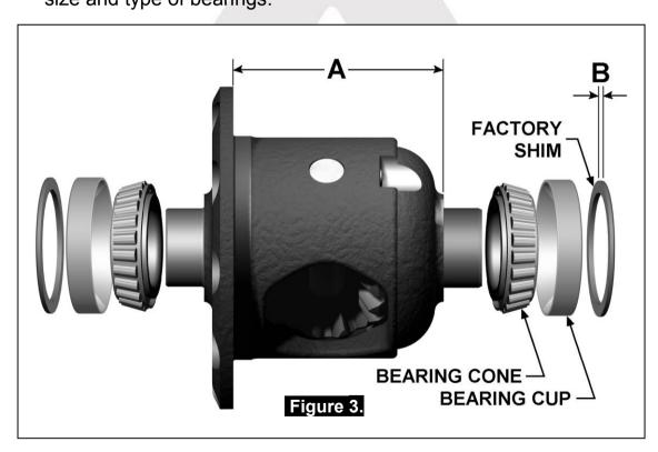
Using a caliper or similarly accurate measurement method (i.e., able to take accurate measurements within 0.04mm [0.0015"]), measure the distance from the shoulder of the bearing journal to the ring gear mounting face (shown as 'A' in Fig.3.) and record this measurement as 'A'.
