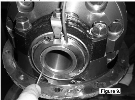
☐ Check that the seal housing is now secured from rotating and that it is still sitting flat against the adjuster nut.
