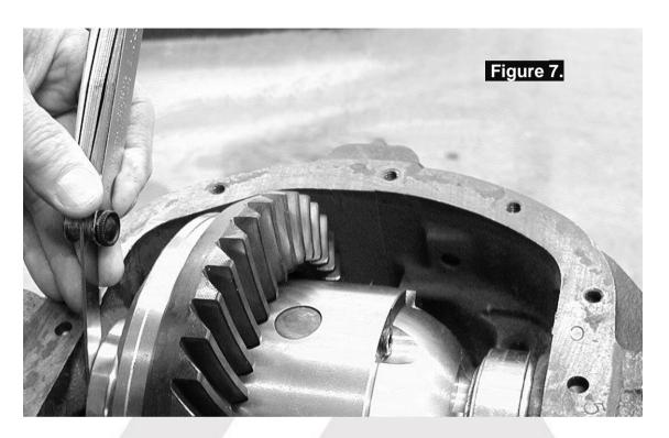
Add the specified preload amount to the end float measurement determined with the feeler gauge to determine a shim amount for 'E' (Refer to Figure 6.).
