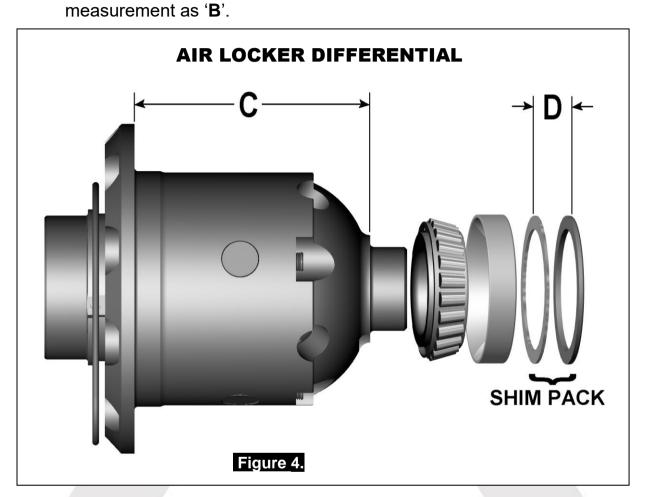
☐ Measure the distance from the *Air Locker* bearing shoulder to the ring gear mounting face (shown as 'C' in Figure 4.) and record this measurement as 'C'.
