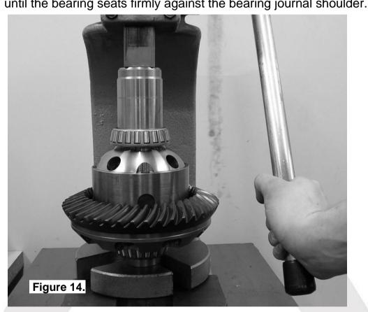
Invert the *Air Locker* and press the other tapered roller bearing cone onto the opposite bearing journal of the differential carrier until the bearing seats firmly against the bearing journal shoulder.
