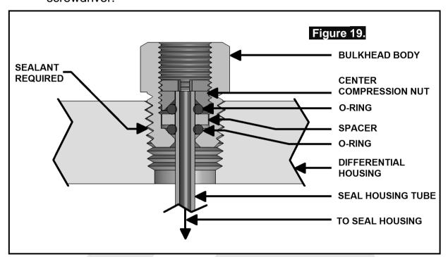
Make sure the seal housing tube is all of the way into the center compression nut while you are tightening it.
