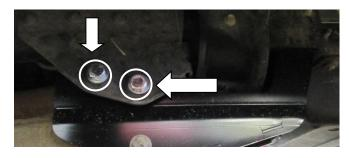
10. Insert top M18 bolt of radius arm on axle end loosely, then lever radius arm into new drop bracket, using original M18 bolt to fix, you may need to push/pull the wheel to get the holes to align the fastener with the mount hole.
