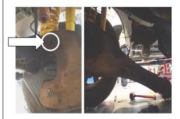
Insert OME radius arm drop bracket, insert both newly supplied M18 x 130mm bolts (6151672) with flat washers and nyloc nut loosely.
