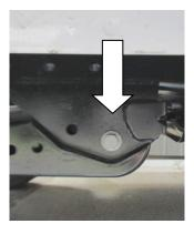
Remove top M18 bolt of radius arm on axle end pivot radius arm to the ground.
