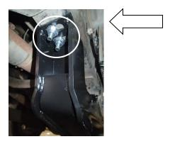
9. Tighten supplied 2 x M18 Bolts and Nyloc nuts on radius arm bracket. Torque to 350Nm (260 lbf.ft)
