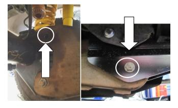
11. Torque 2 x M18 Bolts on the axle end of the radius arm and 1 x M18 bolt on the radius arm fixed end to 350 Nm (260 lbf.ft)
