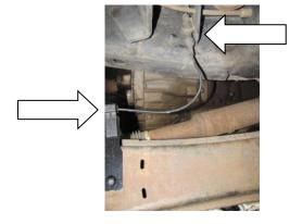
4. CAUTION: The radius arms keep the axle in place underneath the vehicle, at all times at least one of two radius arms must be fully connected. Work only on one side at a time from this step on, failure to do so may event in serious injury.  Where radius arm mounts to vehicle chassis, loosen and remove M18 fastener to disconnect radius arm, you may need to use heat to break down the chemical locking compound.
