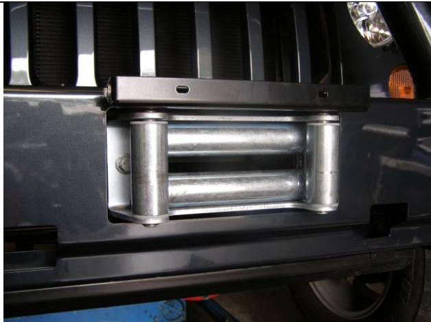
Roller Fairlead installed
