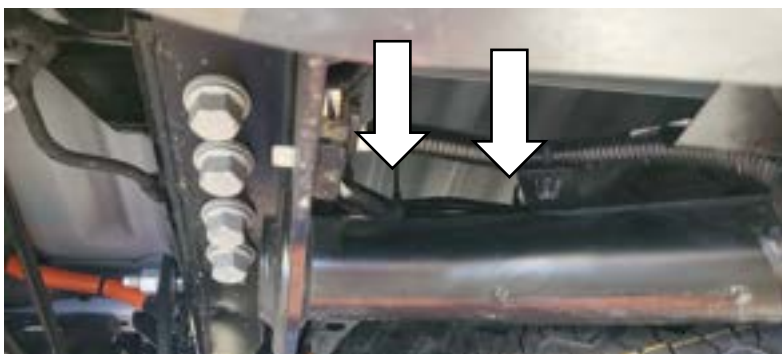
CABLE TIE LOOM ACROSS CHASSIS
