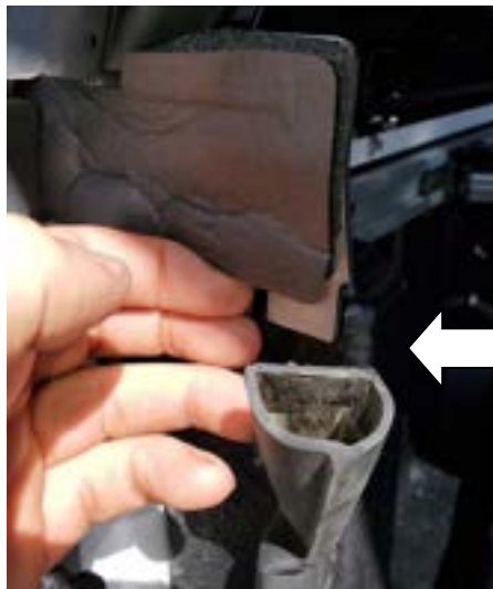
SEAL COMPRESSED TO THREE QUARTER THICKNESS
