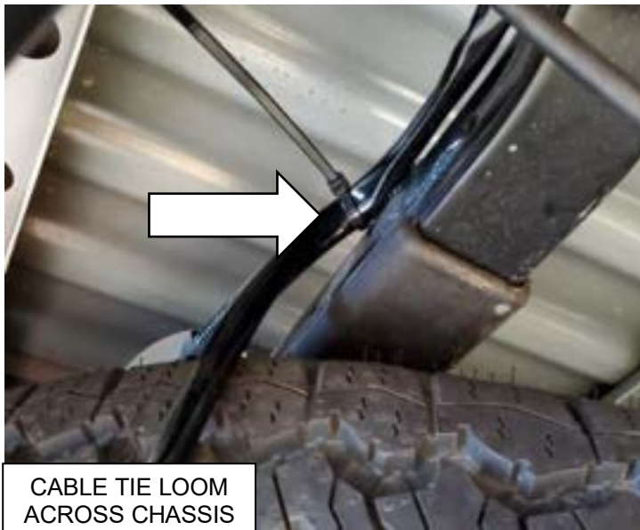
CABLE TIE LOOM AT REAR CORNER OF CHASSIS
