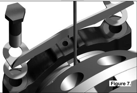
Insert the bearing cap bolts and finger tighten. It is not necessary to torque them down at this time.
