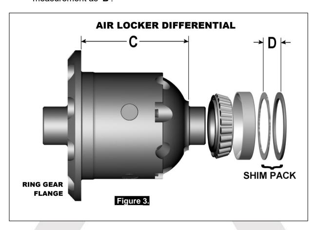
☐ Measure the distance from the *Air Locker* bearing shoulder to the ring gear mounting face (shown as '**C**' in Figure 3.) and record this measurement as '**C**'.
