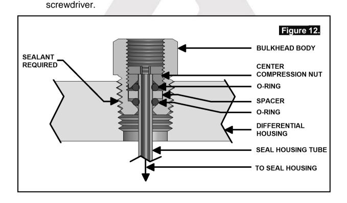
screw it into the bulkhead body, and tighten using Pozidriv #3
