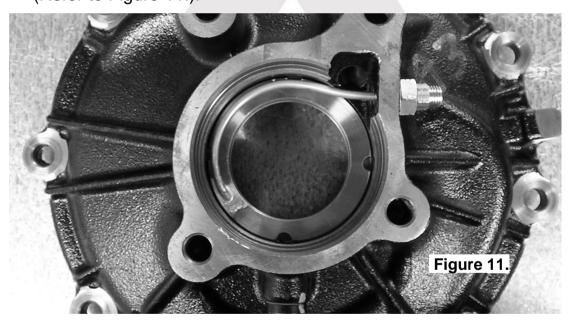
Using a bearing press or arbor press, press the bearing cup into the bottom of the bearing bore until it stops against the seal housing.
