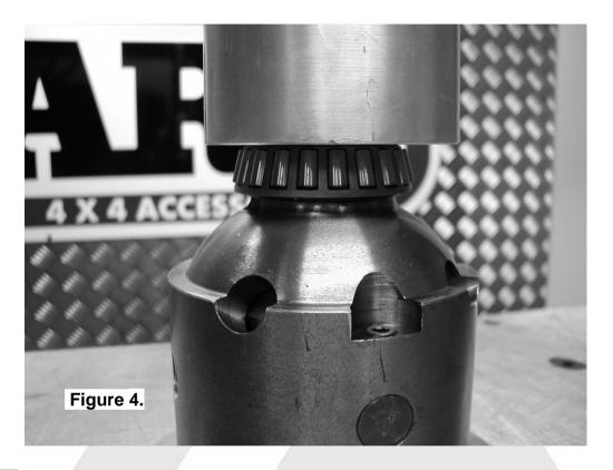
Invert the *Air Locker* and press the second bearing cone onto the bearing journal on the ring gear flange side of the differential (the seal housing side) until the bearing seats firmly against the bearing journal shoulder.
