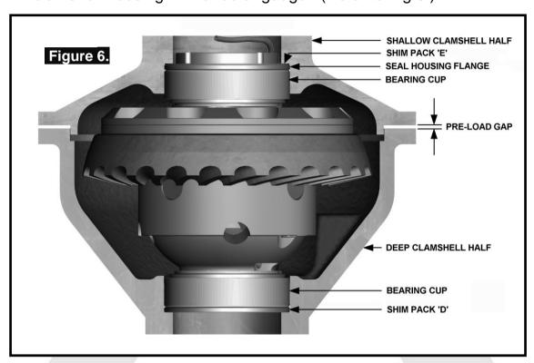
NOTE: The preload gap should be the same when measured all the way around the housing. If this is not true, then reposition the shallow clamshell half and re-measure.
